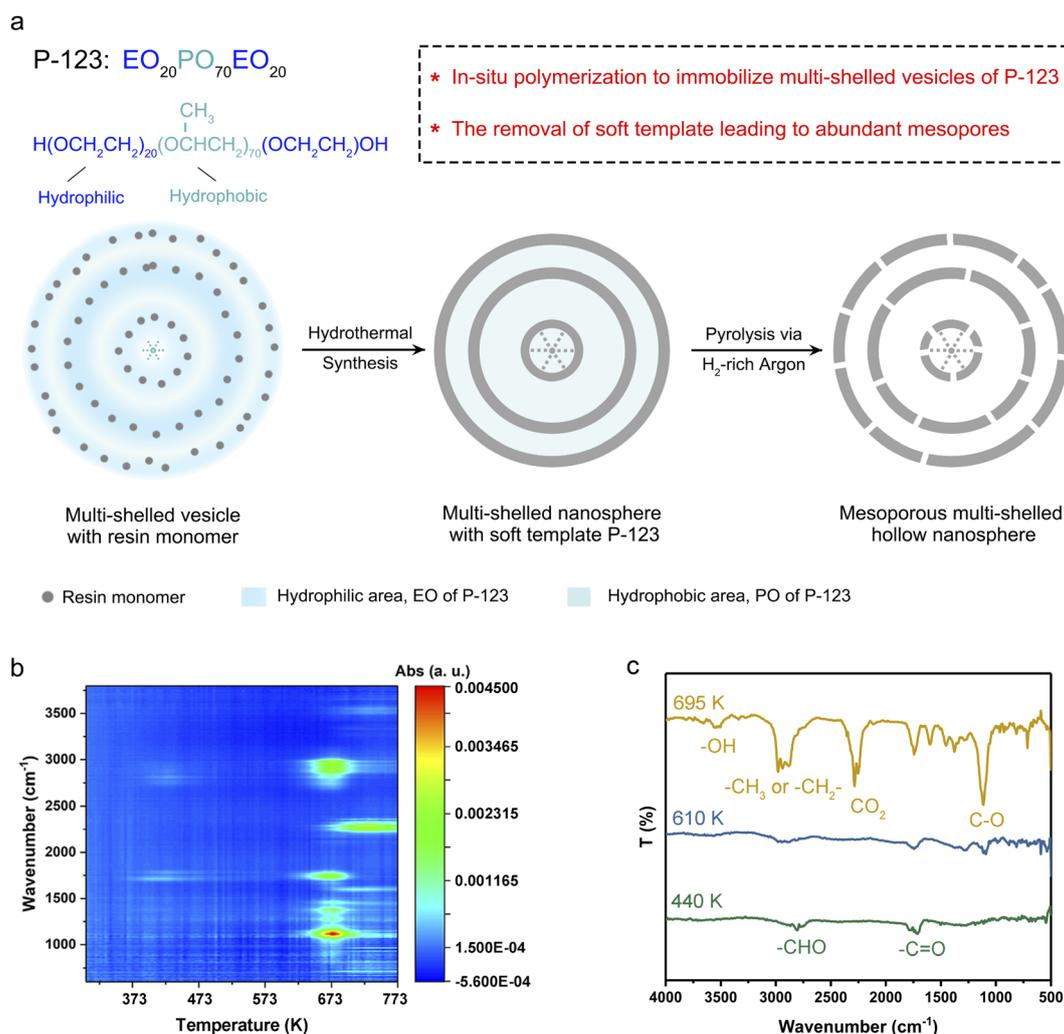
Fig. 1 Synthesis of MsH-MPF-H<sub>2</sub> multi-shelled hollow nanospheres. (a) Schematic illustration of the synthesis program of MsH-MPF-H<sub>2</sub> nanospheres through a template-environment collaboration strategy. (b) Contour diagram of FT-IR spectra for gaseous products of MPF during pyrolysis. (c) FT-IR spectra for gaseous products at different temperatures respectively.
