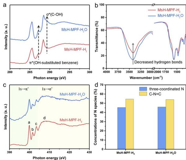
Fig. 3 Atomic structure analysis. (a) Carbon and (c) nitrogen K-edge X-ray absorption near-edge spectroscopy (XANES) of MsH-MPF-H<sub>2</sub> and MsH-MPF-H<sub>2</sub>O nanospheres, respectively. (b) FT-IR spectra of MsH-MPF-H<sub>2</sub> and MsH-MPF-H<sub>2</sub>O nanospheres, respectively. (d) Concentrations of N species in MsH-MPF-H<sub>2</sub> and MsH-MPF-H<sub>2</sub>O according to the X-ray photoelectron spectroscopy (XPS) spectrum.
