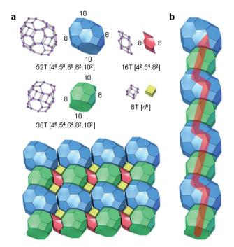
Fig. 2 (a) The tiling presentation of the 2D pore structure of PST-35 and (b) its zig-zag 10-ring channel consisting of strictly alternating 52 T-atom (ptf-1 ([ $4^85^86^88^210^2$ ])) and 36 T-atom (ptf-2 ([ $4^65^46^48^210^2$ ])) cages.
