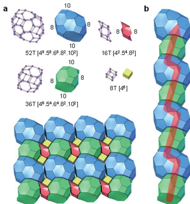
Fig. 2 (a) The tiling presentation of the 2D pore structure of PST-35 and (b) its zig-zag 10-ring channel consisting of strictly alternating 52 T-atom (*ptf-1* ([4<sup>8</sup>5<sup>8</sup>6<sup>8</sup>8<sup>2</sup>10<sup>2</sup>])) and 36 T-atom (*ptf-2* ([4<sup>6</sup>5<sup>4</sup>6<sup>4</sup>8<sup>2</sup>10<sup>2</sup>])) cages.
