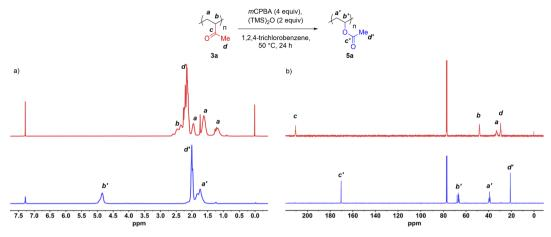
Fig. 3 Exhaustive BV oxidation of commercial PMVK homopolymers. Comparison of (a) <sup>1</sup>H NMR spectra and (b) <sup>13</sup>C NMR spectra before and after exhaustive BV oxidation of commercial PMVK 3a. The NMR spectra were recorded using CDCl<sub>3</sub> as a solvent.
