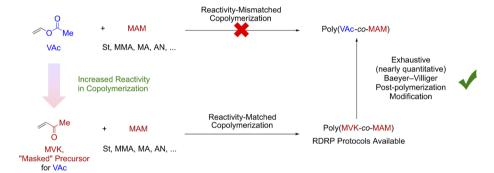
Scheme 1 Accessing synthetically challenging poly(VAc-co-MAM)s with an exhaustive Baeyer-Villiger post-polymerization modification.
