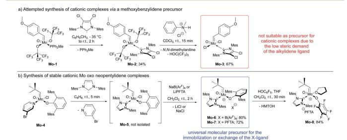
Scheme 1 (a) Synthesis of 4-methoxybenzylidene complexes that could not be further transformed into cationic species; (b) synthesis of cationic molybdenum oxo neopentylidene complexes.
