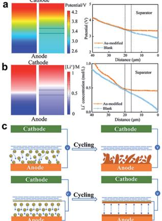
Fig. 3 (a) Simulation modes of electric field values of blank (left) and Au-modified (right) cells in the voltage range from 2.7 to 4.2 V. (b) Simulation results of Li<sup>+</sup> concentration distribution for Li||LFP cells using blank (left) and Au-modified (right) separators. (c) Schematic diagram of Li dendrite growth in batteries based on different separators.
