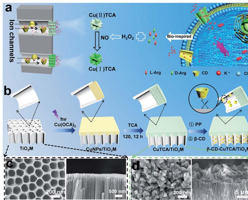
Fig. 1 (a) Schematic illustration of  $\beta$ -CD-CuTCA/TiO<sub>2</sub>M and the principle of the recognition-quantification membrane. (b) Illustration of the preparation of  $\beta$ -CD-CuTCA/TiO<sub>2</sub>M from TiO<sub>2</sub>M. SEM images of the base entrance side and cross-section for (c) TiO<sub>2</sub>M and (d) CuTCA/TiO<sub>2</sub>M.
