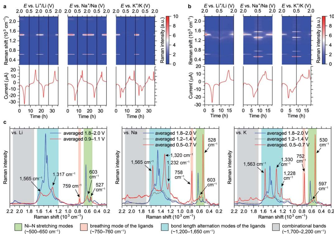
Fig. 4 Evolution of Raman spectra of NiBTA in the 0.5–2.0 V vs.  $M^+/M$  potential ranges: Raman intensity maps and current vs. time (vs. potential) profiles for the measurements with (a) the near-infrared and (b) the green lasers; (c) averaged Raman spectra for selected potential ranges during the initial discharge. The spectra in (c) were measured with the excitation wavelength of 532 nm; characteristic band regions are indicated.
