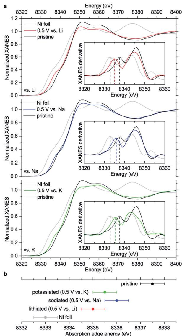
Fig. 6 (a) XANES spectra of NiBTA-based electrodes in pristine and reduced ( $0.5\text{ V vs. M}^+/M$ ) states compared to Ni foil; insets: first derivatives of the XANES spectra; (b) estimated energies of XANES absorption edges. Error bars in (b) are set as halves of the energy increments during the measurement scans, which were  $1\text{ eV}$ .
