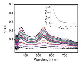
Fig. 2 Transient absorption spectra of 1 in degassed toluene at 298 K at decay times of  $0-4~\mu s$  and the decay trace monitored at 535 nm in
