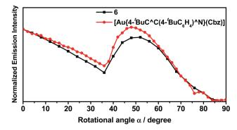
Fig. 6 Angular-dependent PL intensities of the p-polarized light of 6 and  $[Au\{4^-^tBuC^\wedge_6H_4)^\wedge N\}(Cbz)]$  (11% v/v) in m-CBP thin films with 20 nm thickness.
