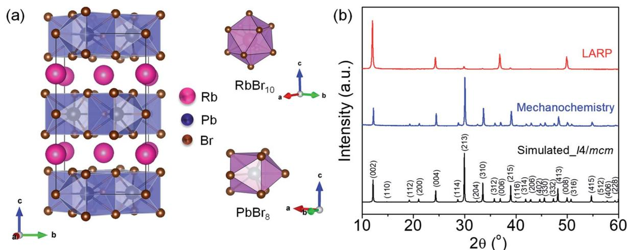
Fig. 1 (a) Crystal structure of  $\text{RbPb}_2\text{Br}_5$  viewed along the crystallographic  $a$ -axis and in the coordination environment of Rb and Pb. (b) PXRD patterns of  $\text{RbPb}_2\text{Br}_5$ , obtained by mechanochemistry and ligand-assisted reprecipitation (LARP) methods.
