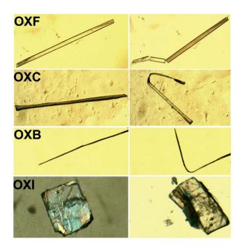
**Fig. 4** The mechanical properties in the oxalate compounds. The OXF crystals are brittle, while OXC and OXB show plastic bending. The block-like crystals of OXI undergo shearing under applied stress.
