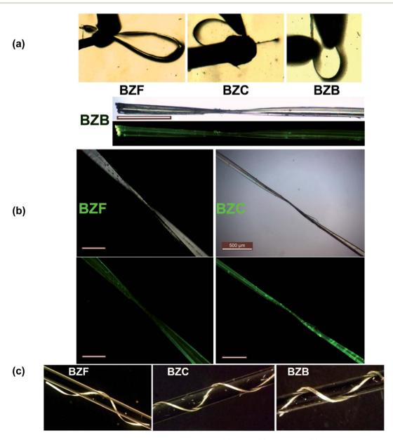
Fig. 1 The crystals of BZF, BZC, and BZB under different deformation stages. (a) Elastic, (b) twisted and (c) coiled around a capillary tube. The scale bar corresponds to 500 µm.
