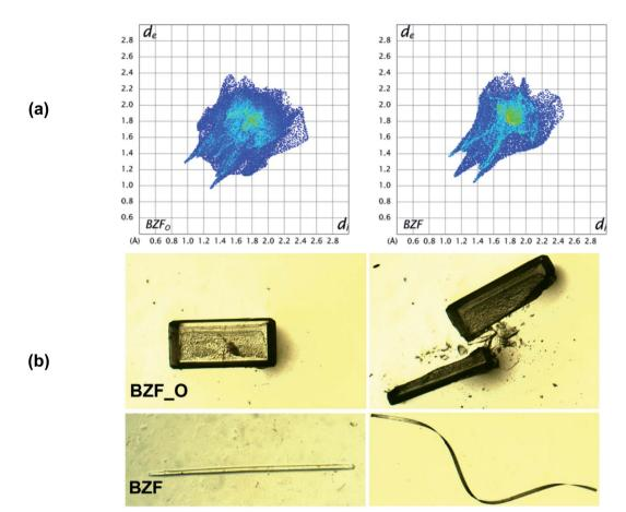
Fig. 2 The dimorphs of the benzil F-derivative (BZF\_O and BZF): (a) HS fingerprint plot highlights the difference in the interaction characteristics; (b) distinct mechanical characteristics of the dimorphs.
