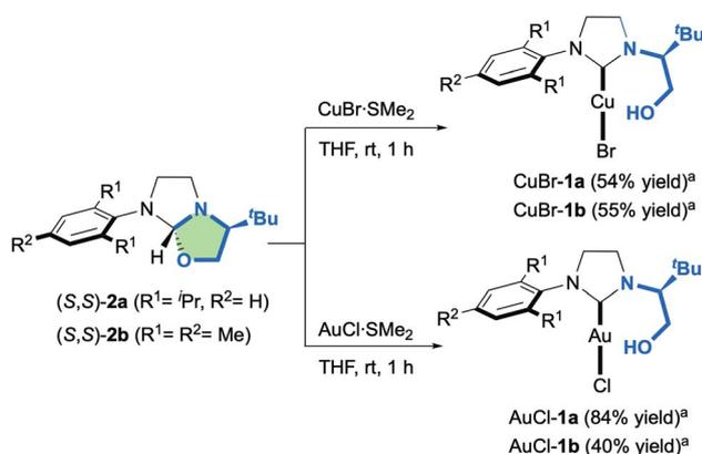
Scheme 3 Synthesis of chiral hydroxyalkyl–NHC CuBr-**1a,b** and AuCl-**1a,b** complexes from oxazolidines **2a,b**. <sup>a</sup>Isolated yields after silica gel filtration.
