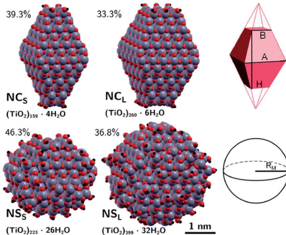
Fig. 9 Top: faceted TiO<sub>2</sub> NPs and a corresponding schematic representation of the Wulff-shape decahedron. Bottom: spherical TiO<sub>2</sub> nanoparticles and a corresponding schematic representation of the sphere. The surface-to-bulk percentage ratio and stoichiometry are also shown. Reprinted with permission from G. Fazio, L. Ferrighi and C. Di Valentin, *J. Phys. Chem. C*, 2015, **119**, 20735–20746. Copyright 2015 American Chemical Society.
