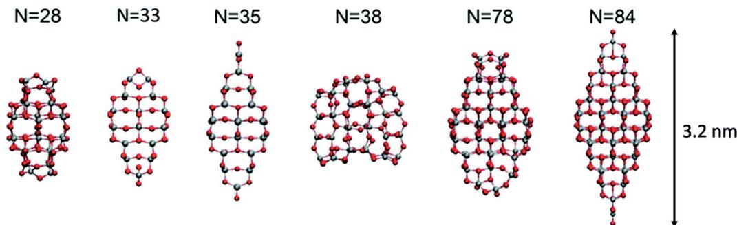
Fig. 2 Atomic structures of the top-down  $(\text{TiO}_2)_n$  nanocrystals investigated in ref. 20. The scale bar on the right strictly refers to the larger model. Titanium, red; oxygen, grey. Reproduced from ref. 20 with permission from the Royal Society of Chemistry.
