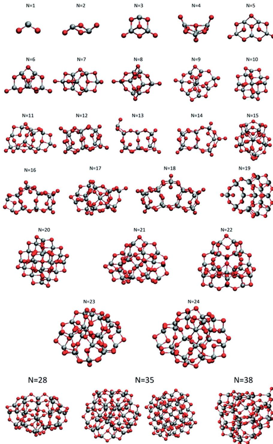
Fig. 1 Atomic structures of the low-energy bottom-up  $(\text{TiO}_2)_n$  nanocrystals investigated in ref. 20. For  $N = 35$ , the structure on the right was obtained by data mining from a tetrahedral  $(\text{CeO}_2)_{35}$  nanoparticle in ref. 22. Titanium, red; oxygen, grey. Reproduced from ref. 20 with permission from the Royal Society of Chemistry.
