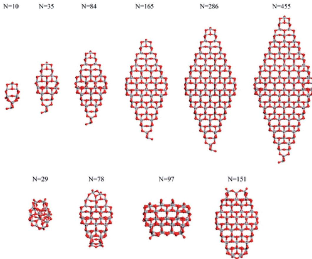
Fig. 4 The octahedral (top) and cuboctahedral (bottom)  $(\text{TiO}_2)_n$  nanoparticles investigated in ref. 21. Reprinted with permission from O. Lamiel-Garcia, K. C. Ko, J. Y. Lee, S. T. Bromley and F. Illas, *J. Chem. Theory Comput.*, 2017, 13, 1785–1793. Copyright 2017 American Chemical Society.
