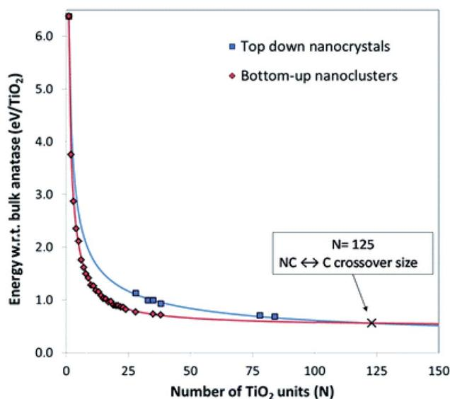
Fig. 3 Energies of bottom-up and top-down  $(\text{TiO}_2)_n$  nanoclusters with the corresponding fitting lines. The NC  $\leftrightarrow$  C crossover size is indicated by the cross at  $n = 125$  (i.e., 375 atoms). Reproduced from ref. 20 with permission from the Royal Society of Chemistry.
