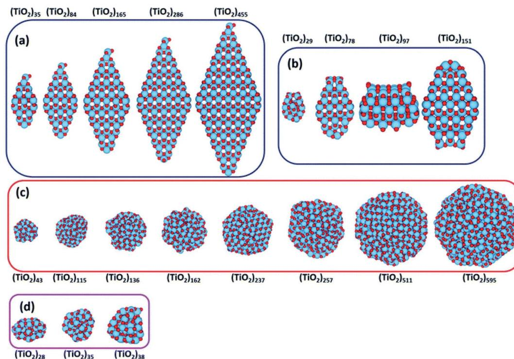
Fig. 6 ( $\text{TiO}_2$ )<sub>n</sub> nanoparticles ( $n = 28$ –595) with (a) bipyramidal, (b) cuboctahedral, and (c) spherical morphologies, and (d) quasi-spherically globally optimised structures investigated in ref. 42. Red/blue spheres correspond to O/Ti atoms. Reproduced from ref. 42 with permission from the Royal Society of Chemistry.
