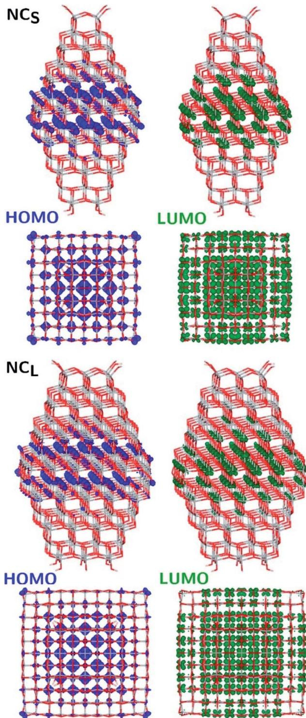
Fig. 10 Side (upper) and top (lower) views of the electronic density plots of the frontier orbitals of  $\text{NC}_5$  and  $\text{NCL}$  (isosurface =  $5 \times 10^{-4}$  au). Reprinted with permission from G. Fazio, L. Ferrighi and C. Di Valentin, *J. Phys. Chem. C*, 2015, **119**, 20735–20746. Copyright 2015 American Chemical Society.
