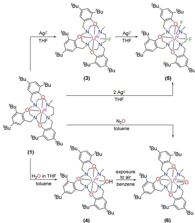
Scheme 2 Synthesis of  $[(\text{cyclen}(\text{Me})(t\text{-Bu},t\text{-BuArO})_3)\text{U}^{\text{IV}}(\text{F})]$  (**3**),  $[(\text{cyclen}(\text{Me})(t\text{-Bu},t\text{-BuArO})_3)\text{U}^{\text{IV}}(\text{OH})]$  (**4**),  $[(\text{cyclen}(\text{Me})(t\text{-Bu},t\text{-BuArO})_3)\text{U}^{\text{V}}(\text{F})_2]$  (**5**), and  $[(\text{cyclen}(\text{Me})(t\text{-Bu},t\text{-BuArO})_3)\text{U}^{\text{V}}(\text{O})]$  (**6**).
