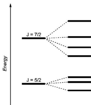
Fig. 4 Schematic energy levels for a 5f<sup>1</sup> system assuming the spin-orbit interaction is greater than the ligand field interaction.<sup>29</sup>
