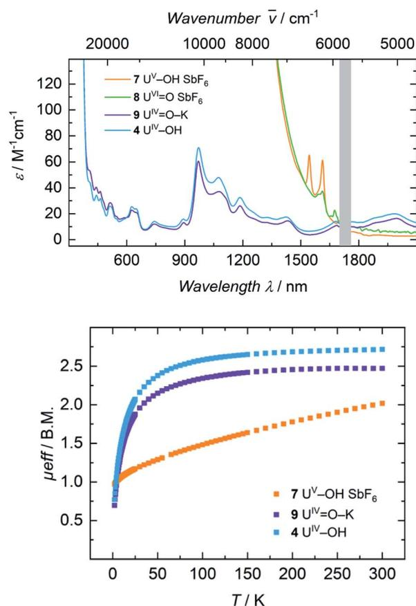
Fig. 8 Top: Electronic absorption spectra of complexes **4**, **7**, **8**, and **9** were recorded at room temperature in benzene (**8**) and THF (**4**, **7**, **9**) solution. Data points from 1700 nm to 1760 nm are omitted due to a detector change from a PbS to an In/Ga/As detector. Bottom: VT SQUID magnetization measurements of microcrystalline, solid samples of **4**, **7** and **9**.
