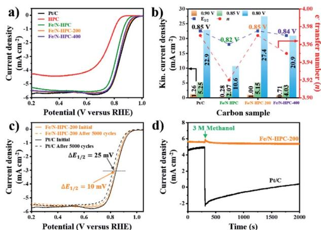
Fig. 6 (a) LSV curves of Pt/C, HPC and Fe/N-HPC, Fe/N-HPC-200 and Fe/N-HPC-400. (b) Electron transfer number,  $E_{1/2}$  and kinetic current density of Pt/C, Fe/N-HPC, Fe/N-HPC-200 and Fe/N-HPC-400. (c) LSV curves of Pt/C and Fe/N-HPC-200 before and after the accelerated durability test (ADT). (d) Chronoamperometric response of Pt/C and Fe/N-HPC-200 with 3 M methanol at 0.65 V and 1600 rpm. All data are obtained in O<sub>2</sub>-saturated 0.1 M KOH electrolyte.
