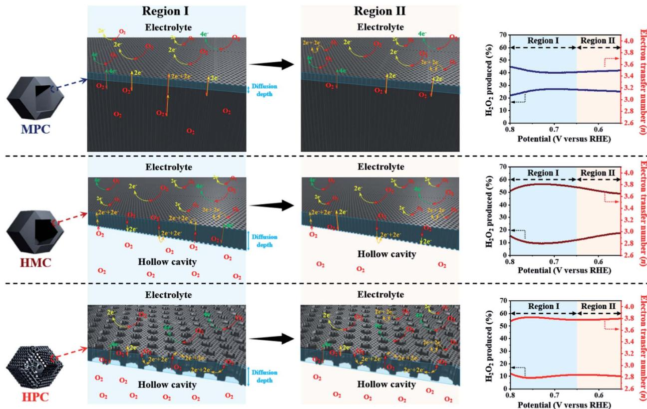
Fig. 4 Graphical description of proposed effect of different nanoarchitectures (MPC, HMC and HPC) on overall electron transfer number calculated from RRDE method ( $4e^-$ ,  $2e^- + 2e^-$  and  $2e^-$  indicate four electron, double two electron and single two electron transfer pathways, respectively).
