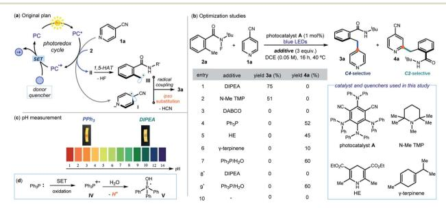
Fig. 2 Initial explorations. (a) Design plan. (b) Optimization studies: reactions performed under argon on a 0.1 mmol scale at 40 °C for 16 h under illumination by a blue LED strip ( $\lambda_{max}$  = 465 nm, 14 W) using 3 equiv. of 1a and additive. Yield determined by <sup>1</sup>H NMR analysis. (c) Measuring the pH of the reaction media. (d) Rationale for the acidity increase in the PPh<sub>3</sub>-based protocol. \*Performed under air.
