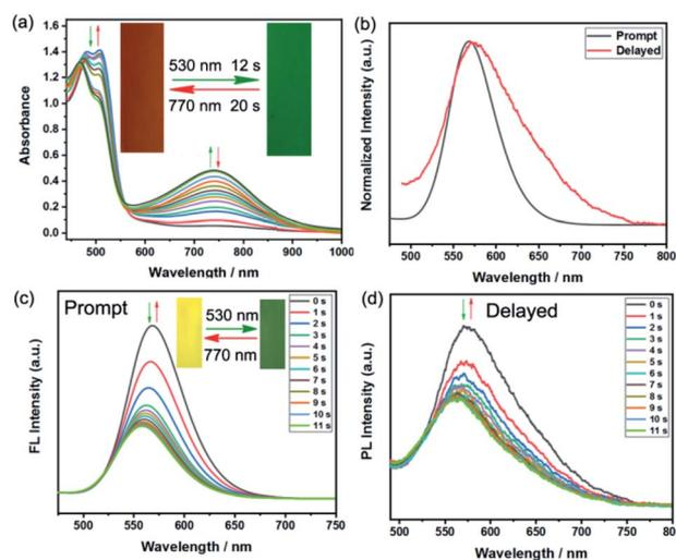
Fig. 4 (a) The absorption spectra of **BFBDT**E in the PMMA film upon alternating irradiation with green and NIR light. Inset: corresponding color changes upon light irradiation. (b) Prompt and delayed fluorescence spectra of **BFBDT**E in the PMMA film. Prompt (c) and delayed (d) fluorescence spectra of **BFBDT**E doped in the PMMA film upon alternating irradiation with green and NIR light ( $\lambda_{\text{ex}} = 450$  nm). Insets: corresponding fluorescence changes upon light irradiation.
