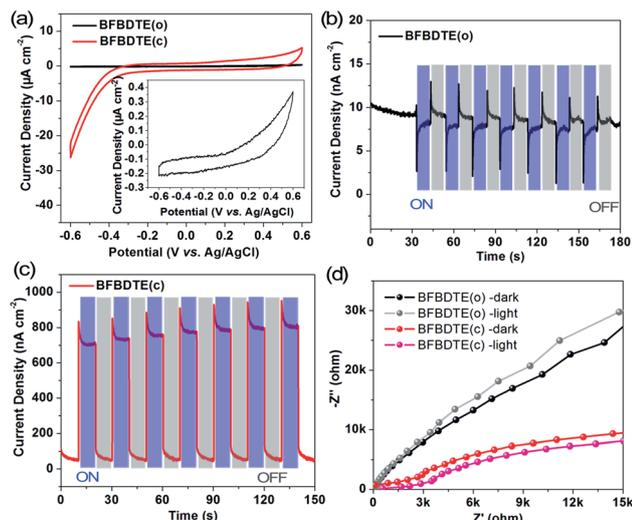
Fig. 5 (a) Cyclic voltammograms of **BFBDTE(o)** and **BFBDTE(c)** measured in 0.5 M  $\text{Na}_2\text{SO}_4$  aqueous solution. Transient current density–time curves of **BFBDTE(o)** (b) and **BFBDTE(c)** (c) without bias potentials. (d) Electrochemical impedance spectroscopy (EIS) Nyquist plots of **BFBDTE(o)** and **BFBDTE(c)** measured at 0 V bias potentials.
