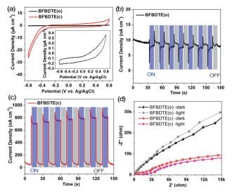
Fig. 5 (a) Cyclic voltammetry curves of BFBDTE(o) and BFBDTE(c) measured in 0.5 M Na<sub>2</sub>SO<sub>4</sub> aqueous solution. Transient current density-time curves of BFBDTE(o) (b) and BFBDTE(c) (c) without bias potentials. (d) Electrochemical impedance spectroscopy (EIS) Nyquist plots of BFBDTE(o) and BFBDTE(c) measured at 0 V bias potentials.
