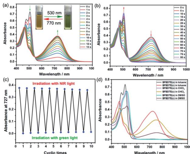
Fig. 2 The absorption spectra changes of **BFBDTE** in toluene ( $2.0 \times 10^{-5} \text{ mol L}^{-1}$ ) upon alternating irradiation with green light at 530 nm (a) and NIR light at 770 nm. (b) The insets show the corresponding color changes upon photoirradiation. (c) The fatigue resistance of **BFBDTE** in toluene for ten cycles. (d) The absorption spectra of **BFBDTE** before and after irradiation with green light in various solvents ( $2.0 \times 10^{-5} \text{ mol L}^{-1}$ ).
