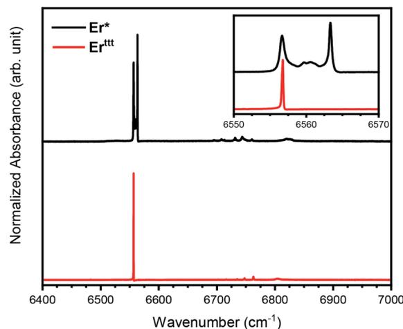
Fig. 5 FTIR absorption spectra of  $\text{Er}^*$  and  $\text{Er}^{\text{tnt}}$  SIMs at 3 K, corresponding to the energy range of the intra-4f transitions from the lowest doublet of the  $^4I_{15/2}$  manifold to the doublets of the excited manifold  $^4I_{13/2}$ . The inset shows a zoom on the sharpest transition lines.
