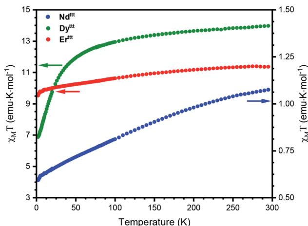
Fig. 2 Temperature dependence of χ<sub>M</sub>T for Er<sup>tBu</sup>, Dy<sup>tBu</sup> and Nd<sup>tBu</sup> measured in the 2–300 K range. χ<sub>M</sub>T values for Er<sup>tBu</sup> and Dy<sup>tBu</sup> were scaled by factors of 1.33 and 1.45 to correct for the errors associated with a small sample mass.
