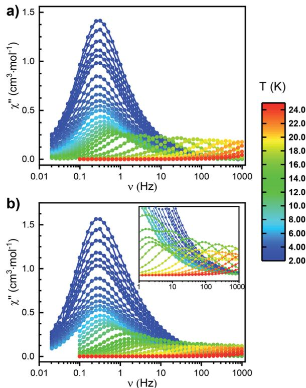
Fig. 4 Frequency dependence of the out-of-phase component of the AC susceptibility measured in zero external DC field between 2 and 24 K for (a)  $\text{Er}^{\text{III}}$  and (b)  $\text{Er}^*$ . Circles represent experimental data points; the lines do not have any physical meaning.
