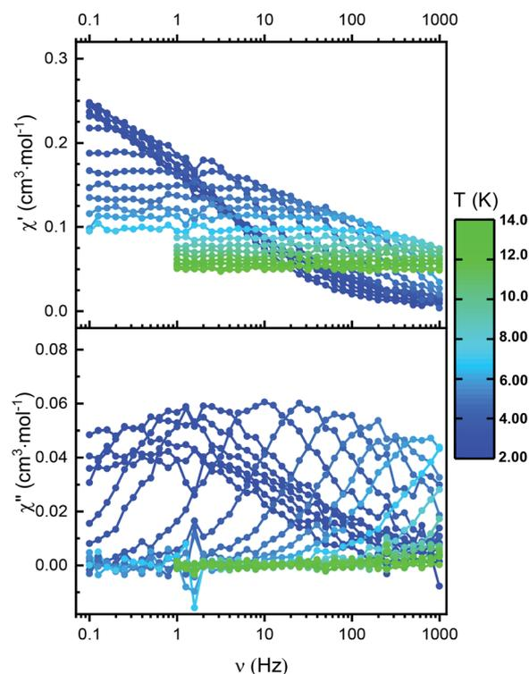
Fig. 6 Frequency dependence of both in-phase (top) and out-of-phase (down) components of the AC susceptibility measured in zero external DC field between 2 and 14 K for  $\text{Nd/Y}^{\text{III}}$ . Circles represent experimental data points; the lines do not have any physical meaning.
