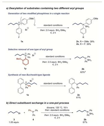
Scheme 3 Further applications. <sup>a</sup>8:1 mixture with 2-methoxybiphenyl.
