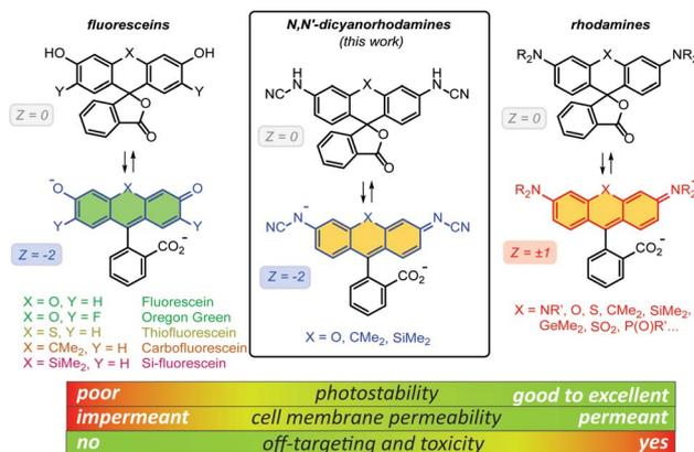
Fig. 1 General chemical structures of fluoresceins, rhodamines and newly designed *N,N'*-dicyanorhodamines and the rationale behind their use in live-cell imaging.
