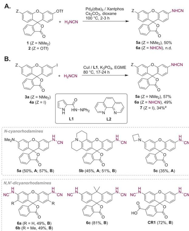
Fig. 2 Synthesis of *N*-cyano- and *N,N'*-dicyanorhodamine fluorophores under Buchwald–Hartwig (A) and Ullmann (B) reaction conditions.<sup>a</sup> Ligand L2 was used instead of L1; EGME – ethylene glycol monomethyl ether.
