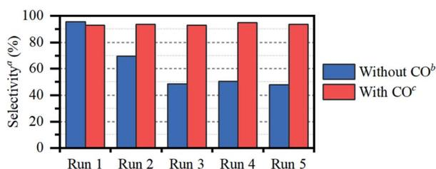
Fig. 1 Preservation of propene over multiple runs. <sup>a</sup>Fraction of propene in the (propene + propane) fraction. Conditions: RuBr<sub>3</sub>·xH<sub>2</sub>O (2 mol%), propene (1 bar), Bu<sub>4</sub>PBr (577 mg, 3.4 mmol). Pretreatment: CO gas (1 bar) 40 bar H<sub>2</sub>, 0.5 h, 180 °C. Each hydrogenation uses a fresh charge of propene gas (1 bar), 40 bar H<sub>2</sub>, 1 h, 220 °C. <sup>b</sup>CO pretreatment before first run. <sup>c</sup>CO pretreatment before each run.
