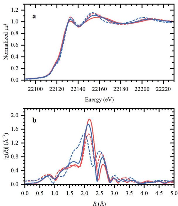
Fig. 3 XANES (a) and magnitudes of Fourier-transformed ( $4$ - $15 \text{ \AA}^{-1}$ ) phase-uncorrected FT-EXAFS (b) data for  $[\text{RuBr}_2(\text{CO})_3]_2$  (red) and  $[\text{RuCl}_2(\text{CO})_3]_2$  (blue), before (dashed lines) and after (solid lines) dissolution in  $\text{Bu}_4\text{PBr}$ .
