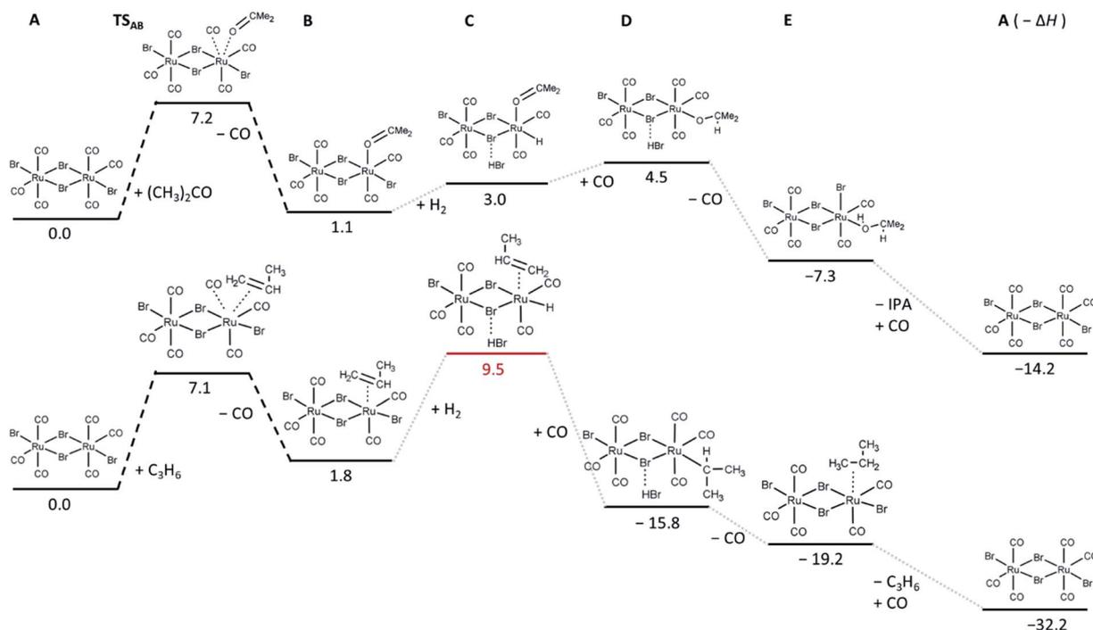
Fig. 8 Relative energies in  $\text{kcal mol}^{-1}$  of the most stable intermediates and first transition state determined for acetone (top) and propene (bottom) hydrogenation reactions. The corresponding relaxed structures and output files are attached in ESI.†
