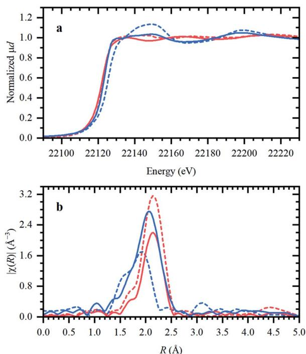
Fig. 2 XANES (a) and magnitudes of Fourier-transformed (4–15 Å<sup>-1</sup>) phase-uncorrected FT-EXAFS (b) data for RuBr<sub>3</sub> (red) and RuCl<sub>3</sub> (blue), before (dashed lines) and after (solid lines) dissolution in Bu<sub>4</sub>PBr.
