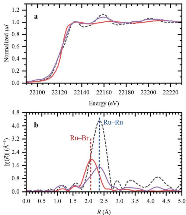
Fig. 6 XANES (a) and phase-uncorrected FT-EXAFS (b) data for  $\text{RuBr}_3$  salt dissolved in IL before (solid red) and after (solid purple) reaction with propene. Dashed grey lines correspond to metallic Ru reference.
