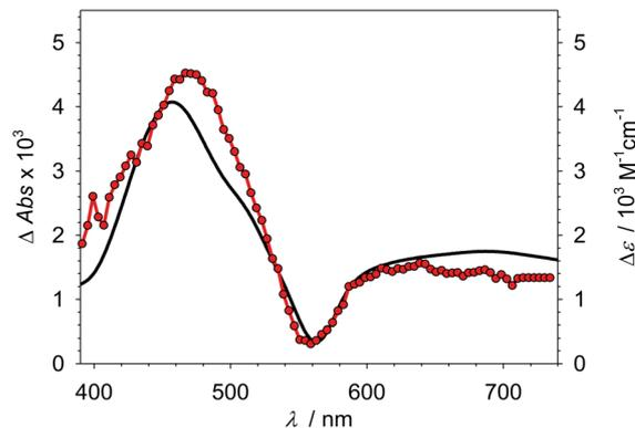
**Fig. 2** Absorption changes upon laser flash excitation (490 nm) of  $[\text{Fe}(\text{III})(\text{btz})_3](\text{PF}_6)_3$  **1** in MeCN : MeOH (4 : 3) with TEA (0.29 M) (●) and difference spectrum between  $[\text{Fe}(\text{III})(\text{btz})_3](\text{PF}_6)_3$  **1** and  $[\text{Fe}(\text{II})(\text{btz})_3](\text{PF}_6)_2$  **2** (–□–).
