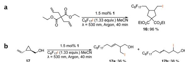
**Scheme 6** Radical (a) ring-closing of diethyl 2,2-diallylmalonate and (b) ring-opening of *trans*-(2-vinylcyclopropyl)methanol *via* the oxidative quenching route of the visible light-mediated ATRA reaction with **1**.
