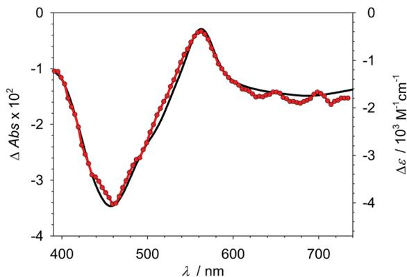
Fig. 3 Absorption changes 50 ns after laser flash excitation (650 nm) of [Fe(II)(btz)<sub>3</sub>](PF<sub>6</sub>)<sub>2</sub> **2** in MeCN : MeOH (4 : 3) with C<sub>8</sub>F<sub>17</sub>I (0.45 M) (●) and difference spectrum between [Fe(II)(btz)<sub>3</sub>](PF<sub>6</sub>)<sub>2</sub> **2** and [Fe(III)(btz)<sub>3</sub>](PF<sub>6</sub>)<sub>3</sub> **1** (1–2, ▴).
