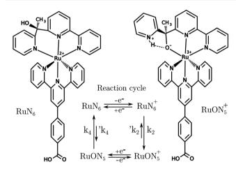
Fig. 5 Structures of RuN<sub>6</sub>, [Ru(HOOC–Ph-tpy)(1-[6-(2,2'-bipyridyl)]-1-(2-pyridyl)ethanol)]<sup>2+</sup>, and RuON<sub>5</sub><sup>+</sup> with related reaction cycle of the electron transfer induced isomerization.  $k_2$  and  $k_4$  are ca. 150–200 and 500–1000 s<sup>-1</sup>, respectively (e<sup>-</sup> transfers occur in ca. 10<sup>4</sup> s).<sup>39</sup>
