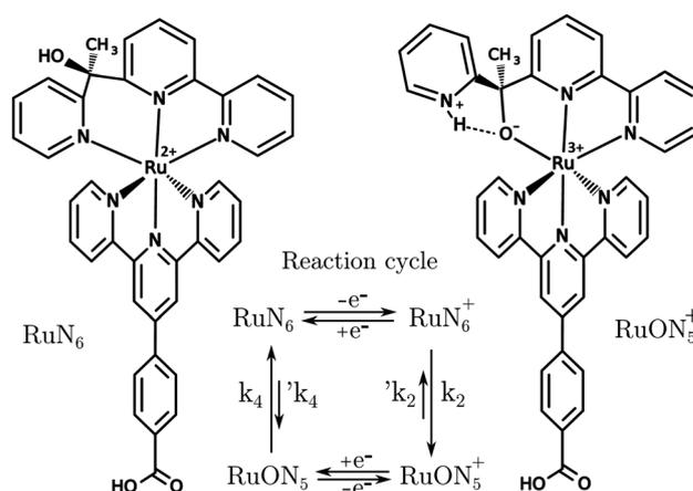
Fig. 5 Structures of RuN<sub>6</sub>, [Ru(HOOC-Ph-tpy)(1-[6-(2,2'-bipyridyl)]-1-(2-pyridyl)ethanol)]<sup>2+</sup>, and RuON<sub>5</sub><sup>+</sup> with related reaction cycle of the electron transfer induced isomerization. *k*<sub>2</sub> and *k*<sub>4</sub> are *ca.* 150–200 and 500–1000 s<sup>-1</sup>, respectively (e<sup>-</sup> transfers occur in *ca.* 10<sup>-4</sup> s).<sup>39</sup>
