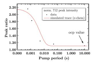
Fig. 9 Comparison of the experimental amplitude ratio of the normalized 712 peaks over time and its simulated trace (as a first order reaction) of the measured kinetics (200 s $^{-1}$ ).
