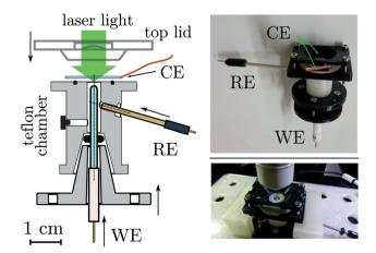
Fig. 4 (Left) Section of the e-chem cell design (Teflon made), see Fig. S1 in ESI,† for detailed technical sketches. The WE and RE electrodes are shown in the final positions, for clarity the CE is not attached to the cell. Supporting flanges for closure are not shown. (Right) Pictures of the real cell.
