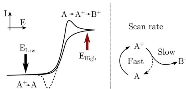
Fig. 1 Schematic cyclic voltammogram of the A/A<sup>+</sup>/B<sup>+</sup> system described in the text, in dashed lines the response obtained at scan-rates able to outcompete reaction A<sup>+</sup> → B<sup>+</sup>. An “infinite pool” of the A species is assumed. On the right, the reaction scheme in function of scan-rates, fast vs. slow.
