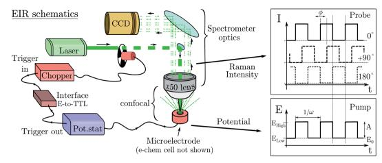
Fig. 2 Scheme of the EIR setup with example of the modulation of Raman intensity and potential vs. time. Only the parts shown in RED are added to a usual Raman spectrometer to implement EIR. In the graphs,  $\phi$  indicates the possibility to shift the phase of the Raman modulation (0°/90°/180°) with respect to the potential SW.
