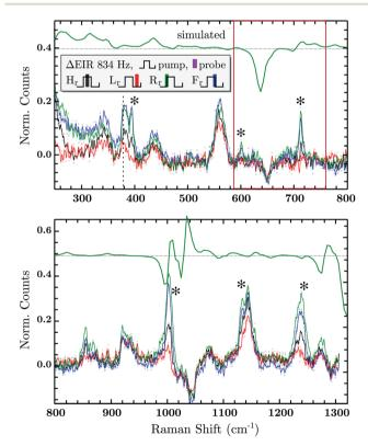
Fig. 8 Difference EIR spectra of the  $RuN_6$  functionalised AuNP electrode of the 834 Hz measurement in all four phase shifts, the ocp spectrum has been taken as reference (subtracted and normalized). EIR phases:  $H_r$  black,  $L_r$  red,  $R_r$  green,  $F_r$  blue. The  $R_r$  trace from numerical simulation is reported in green, shifted for clarity. Discussed spectral range has been highlighted for clarity.
