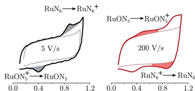
Fig. 6 Electrochemistry of RuN<sub>6</sub> grafted on Pt microelectrode, at two scan-rates 5 and 200 V s<sup>-1</sup>. In dashed lines the blank electrochemistry (without complex) to account for the coulombic current. The grey areas indicate the irreversible waves due to the stable species; the red areas indicates the redox waves due to the unstable species, visible only at high scan-rates.
