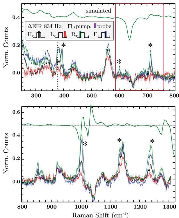
Fig. 8 Difference EIR spectra of the  $\text{RuN}_6$  functionalised AuNP electrode of the 834 Hz measurement in all four phase shifts, the ocp spectrum has been taken as reference (subtracted and normalized). EIR phases:  $H_r$  black,  $L_r$  red,  $R_r$  green,  $F_r$  blue. The  $R_r$  trace from numerical simulation is reported in green, shifted for clarity. Discussed spectral range has been highlighted for clarity.
