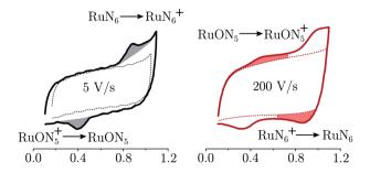
Fig. 6 Electrochemistry of  $RuN_6$  grafted on Pt microelectrode, at two scan-rates 5 and  $200 \text{ V s}^{-1}$ . In dashed lines the blank electrochemistry (without complex) to account for the coulombic current. The grey areas indicate the irreversible waves due to the stable species; the red areas indicates the redox waves due to the unstable species, visible only at high scan-rates.
