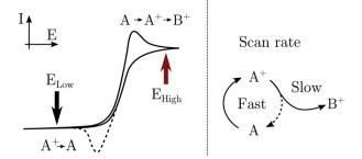
Fig. 1 Schematic cyclic voltammogram of the A/A+/B+ system described in the text, in dashed lines the response obtained at scanrates able to outcompete reaction  $A^+ \rightarrow B^+$ . An "infinite pool" of the A species is assumed. On the right, the reaction scheme in function of scan-rates, fast vs. slow.
