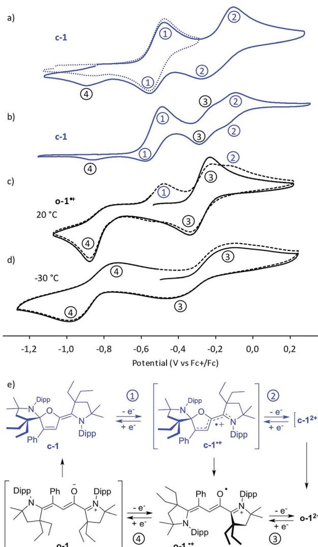
Fig. 3 Cyclic voltammetry at  $100$   $\text{mV s}^{-1}$  rate (if not otherwise stated) with  $0.1$  M  $n\text{Bu}_4\text{NPF}_6$  electrolyte of acetonitrile solution ( $1$  mM) of: (a)  $\mathbf{c}\text{-1}$ , (b)  $\mathbf{c}\text{-1}$  at a rate of  $10$   $\text{mV s}^{-1}$ , (c)  $\mathbf{o}\text{-1}^{\cdot+}$  at  $20$   $^{\circ}\text{C}$ , and (d)  $\mathbf{o}\text{-1}^{\cdot+}$  at  $-30$   $^{\circ}\text{C}$ ; (e) corresponding electrochemical processes.
