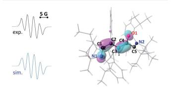
Fig. 2 Left, experimental X-band EPR spectra of 1' in acetonitrile at room temperature (black); the corresponding simulated spectra (blue) with the following set of parameters: line-broadening parameter lw = 0.288 and hyperfine coupling constants  $a(^{14}N) = 11.4$  MHz and  $a(^{1}H) = 10.1$  MHz. Right, representation of computed SOMO.
