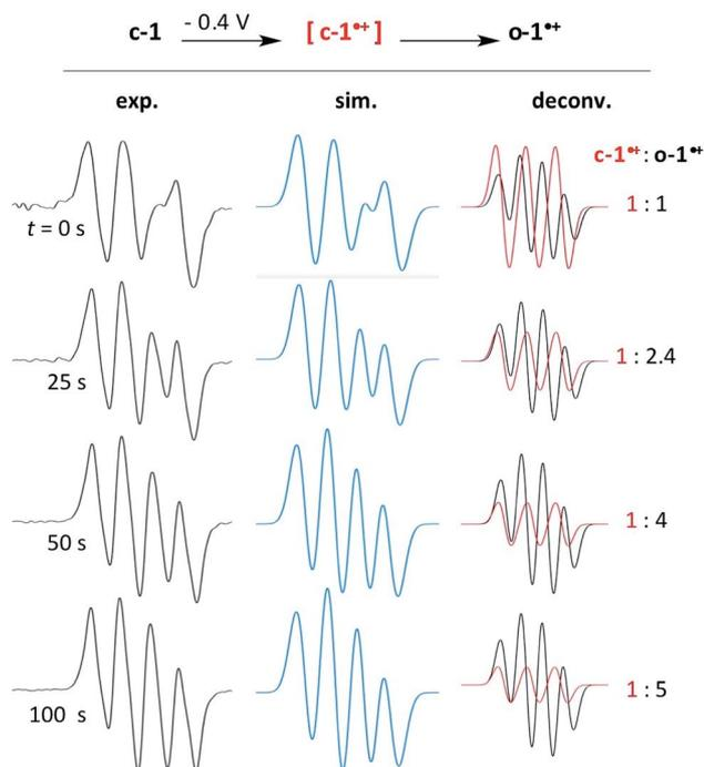
Fig. 4 Left, EPR monitoring of the electrolysis at  $-0.4$  V of **c-1** in acetonitrile; middle, the corresponding simulated spectra; right, deconvolution and respective contribution of **c-1** $\cdot^+$  (red) and **o-1** $\cdot^+$  (black) radicals to the spectra.
