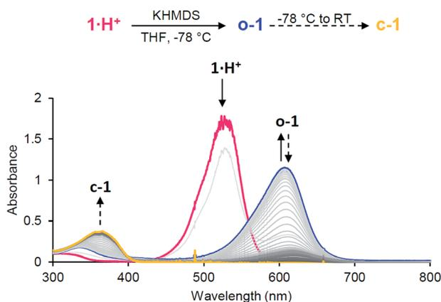
Fig. 5 UV-monitoring of the addition of KHMDS to **1** $\cdot\text{H}^+$  in THF.
