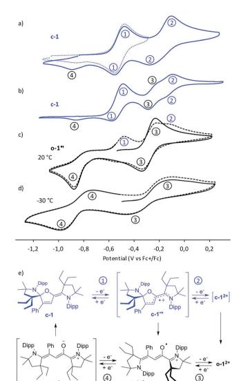
Fig. 3 Cyclic voltammetry at 100 mV s $^{-1}$  rate (if not otherwise stated) with 0.1 M nBu<sub>4</sub>NPF<sub>6</sub> electrolyte of acetonitrile solution (1 mM) of: (a) c-1, (b) c-1 at a rate of 10 mV s $^{-1}$ , (c) o-1 $^{\cdot +}$  at 20 °C, and (d) o-1 $^{\cdot +}$  at -30 °C; (e) corresponding electrochemical processes.
