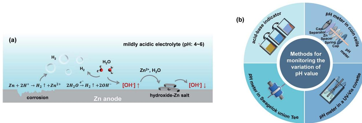
Fig. 3 (a) Schematic illustrations of the reactions under an unstable pH environment at the vicinity of Zn anodes. (b) *In situ* pH monitoring methods for aqueous Zn batteries.
