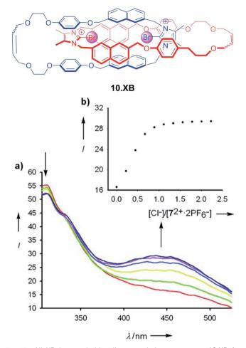
Fig. 13 All-XB bromo-imidazolium-napthalene catenane 10.XB for fluorescent halide sensing. (a) Emission spectra of 10  $\mu$ M 10.XB upon addition of Cl $^-$  in ACN. (b) The corresponding response isotherm at 445 nm. Reproduced with permission from ref. 122 copyright 2011 Wiley.
