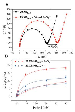
Fig. 34 (A) Capacitive Nyquist plots of  $29.XB_{SAM}$  in the absence and presence of 50 mM  $ReO_4^-$  showing an increased capacitance in the presence of bound anion. (B) Relative capacitive sensor response of  $29.XB_{SAM}$  (filled symbols) and  $29.HB_{SAM}$  (empty symbols) in response to  $ReO_4^-$  (red) and  $I^-$  (blue). Reproduced from ref. 162 with permission of the Royal Society of Chemistry.
