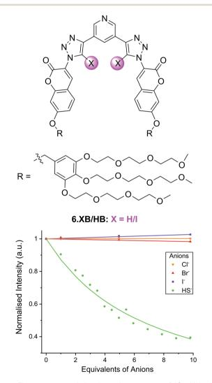
Fig. 11 Fluorescence emission intensity response of 10 μM hydrosulfide-selective coumarin-containing 6.XB in the presence of 10 equiv. of various anions in 10 mM HEPES buffer (pH = 7.4). Reproduced from ref. 101 under the terms of the CC BY license.
