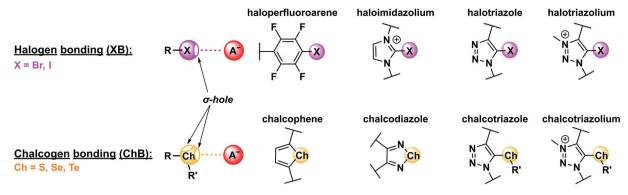
Fig. 2 Schematic depiction of halogen (XB) and chalcogen bonding (ChB) interactions with an anion as archetypical Lewis base. Shown are also commonly employed XB and ChB donor motifs.
