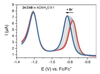
Fig. 27 SWVs of telluroviologen ChB sensor **24.ChB** in ACN/ $\rm H_2O$  9 : 1 upon addition of up to 50 mM Br $^-$ . Only the first reductive couple is responsive, indicative of complete ChB deactivation upon monoreduction. Reproduced with permission from ref. 62 copyright 2022 American Chemical Society.
