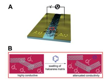
Fig. 36 (A) Schematic depiction of a chemiresistive sensor based on a carbon nanotube matrix between two gold electrodes. (B) Incorporation of haloaryl XB selectors into the sensor matrix enables sensing of pyridine vapours by recognition-induced swelling of the matrix and an associated decrease in conductance. Reproduced with permission from ref. 171 copyright 2016 American Chemical Society.
