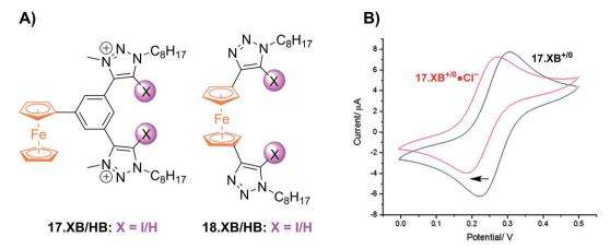
Fig. 21 (A) Chemical structures of the first XB ferrocenyl voltammetric anion sensors. (B) CVs of 17.XB in ACN in the absence (black) and presence of 10 equiv. Cl<sup>-</sup> (red). Adapted from ref. 141 with permission from the Royal Society of Chemistry.
