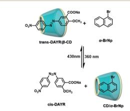
Fig. 1 Schematic illustration of photo-controlled reversible RTP pseudorotaxane in aqueous solutions.
