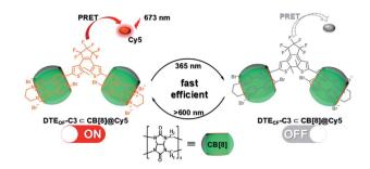
Fig. 13 Schematic illustration of the construction of photocontrolled supramolecular phosphorescence energy transfer based on the diarylethene-modified bromophenylpyridinium salt.
