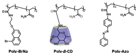
Fig. 3 Schematic illustration of construction of the compound structure of the photoresponsive supramolecular RTP gel based on  $\beta$ -CD and bromonaphthalene.
