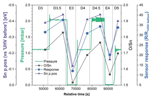
Fig. 7 Correlation between O/Sn ratio of the lattice component (V<sub>O</sub> concentration), Sn p.pos relative to 'UHV before' (band bending) and the sensor response under dynamically changing O<sub>2</sub> pressure conditions during final stages of experiment HIGH\_T. The initial steps were omitted due to the anomalous resistance measurements recorded during steps E1 and E2.
