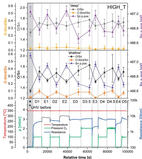
Fig. 5 Results of phenomenological (bottom) and XPS (middle and top) investigation during experiment HIGH\_T. The 'shallow' and 'deep' plots present quantification of XPS spectra with 2.5 and 5 nm sampling depth, respectively. Sn p.pos denotes the binding energy position of the Sn 3d<sub>5/2</sub> peak.
