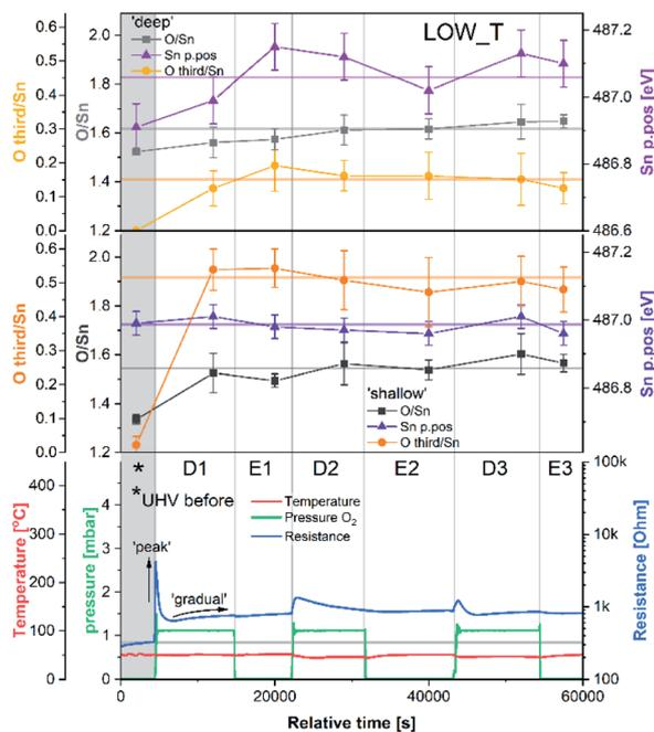
Fig. 2 Results of phenomenological (bottom) and XPS (middle and top) investigation during experiment LOW\_T. The 'shallow' and 'deep' plots present quantification of XPS spectra with 2.5 and 5 nm sampling depth, respectively. Sn p.pos denotes the binding energy position of the Sn 3d<sub>5/2</sub> peak.
