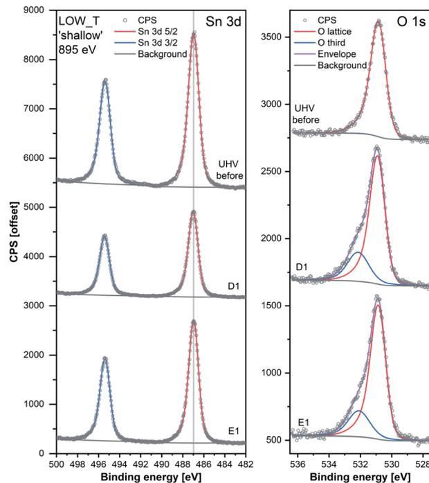
Fig. 3 Comparison of Sn 3d and O 1s high-resolution spectra collected during steps 'UHV before', D1 and E1 of experiment LOW\_T. Peaks were offset along the Y-axis. The lower signal intensity of Sn during D1 compared to the UHV steps is attributable to the attenuation of photoelectrons by the O<sub>2</sub> gas present during that step. The O 1s peaks were normalised with respect to their corresponding Sn 3d peak areas.
