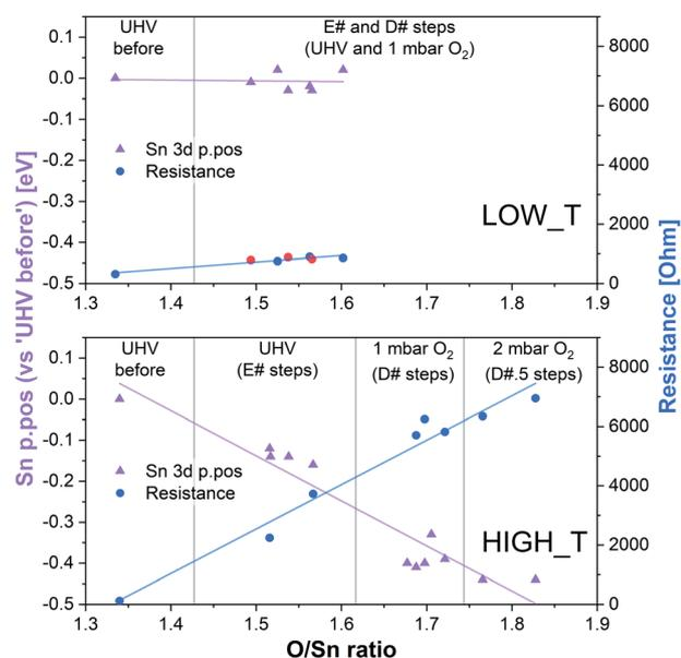
Fig. 4 Summary of band bending (Sn 3d p.pos) and resistance change as a function of oxygen vacancy density in the near surface region derived from the LOW\_T and HIGH\_T experiments. In the LOW\_T plot, the red resistance data points correspond to E# steps. In the HIGH\_T plot, the 'anomalous' resistance data were omitted; for details, see the discussion of the HIGH\_T experiment below and ESI†.
