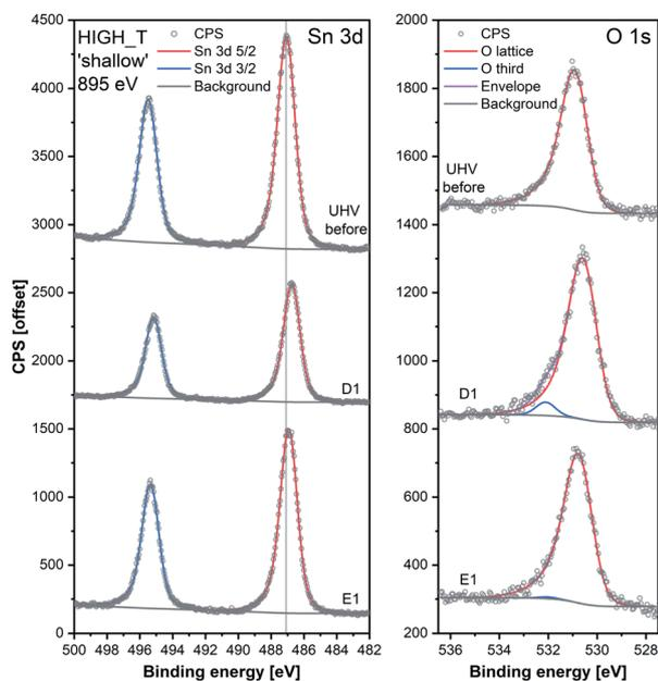
Fig. 6 Comparison of Sn 3d and O 1s high-resolution spectra collected during steps ‘UHV before’, D1 and E1 of experiment HIGH\_T. Peaks were offset along the Y-axis. The lower signal intensity of Sn during D1 compared to the UHV steps is attributable to the attenuation of photoelectrons by the O<sub>2</sub> gas present during that step. The O 1s peaks were normalised with respect to their corresponding Sn 3d peak areas.
