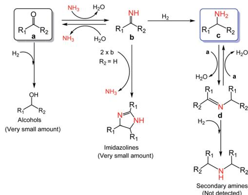
Fig. 5 Proposed mechanism for the reductive amination of carbonyl compounds to primary amines using NH<sub>3</sub> and H<sub>2</sub> over Co@C-N(800).
