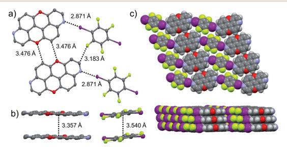
Fig. 11 Single-crystal X-ray structure of co-crystal 3,9-N,N-PXX DITFB. ORTEP representation and structure of four molecules engaging into Hbonds and XBIs (a) organised in supramolecular multi-layered  $\pi-\pi$  stacked (b) sheets (c). Space groups:  $P\overline{1}$ . Atom colours: red O, blue N, purple I, green F, grey C, white H.
