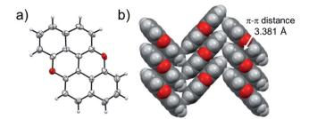
Fig. 7 Single-crystal X-ray structure of PXX. ORTEP representation (a) and (b) herringbone-type arrangement. Space groups:  $P2_1/c$ . Data taken from literature. <sup>52</sup> Atom colours: red O, grey C, white H.
