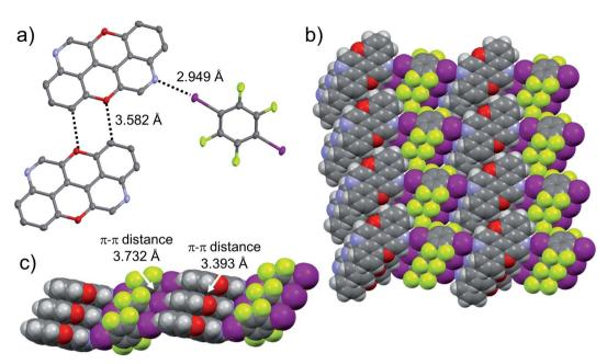
Fig. 12 Single-crystal X-ray structure of co-crystal 4,10-N,N-PXX·DITFB. ORTEP representation and structure of three molecules engaging into H-bonds and XBIs (a) organised in supramolecular  $\pi$ - $\pi$  stacked (b) supramolecular polymers (c). Space groups:  $P\overline{1}$ . Atom colours: red O, blue N, purple I, green F, grey C, white H.
