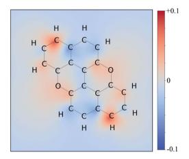
Fig. 3 Excitation charge redistribution map for PXX. This is the excited state CHELPG charges minus ground state CHELPG charges of PXX interpolated over the atomic positions on the  $\sigma$ -scaffold, with the blue and red area indicating the electron depletion and accumulation regions respectively. The colour map ranges from +0.1 (red, donors) to -0.1 (blue, acceptors) electrons.
