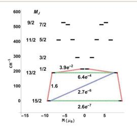
Fig. 11 Blocking diagram from CASSCF(9,7)/QDPT/SINGLE\_ANISO calculations for 5-Er. Blue lines correspond to Orbach relaxation mechanisms, green lines correspond to quantum tunneling of magnetisation, and red lines correspond to the most likely pathway.
