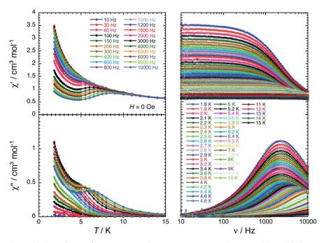
Fig. 6 In-phase (top) and out-of-phase (bottom) components of the molar ac magnetic susceptibility of **3-Dy** measured as a function of temperature at different frequencies (left) and as a function of frequency at different temperatures (right) in zero dc-field. The solid lines on the left plots are a guides for the eye. The solid lines on the right plots are the generalized Debye fits<sup>71,72</sup> of the experimental ac susceptibility data (open dots).
