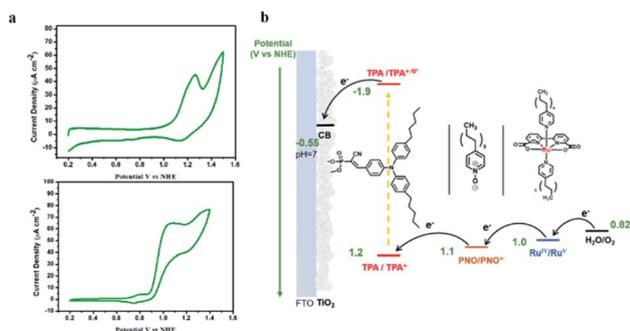
Fig. 7 (a) Cyclic voltammograms of nanoITO|TPA in pH 7, 0.1 M phosphate buffer (top) and catalyst **1** (1 mM) in mixed  $\text{CH}_3\text{CN}/\text{H}_2\text{O}$  (v/v = 1 : 2) solution (bottom) with a scan rate of  $20 \text{ mV s}^{-1}$ . (b) Schematic energy diagram for  $\text{TiO}_2|\text{TPA}|\text{PNO}|\mathbf{1}$ .
