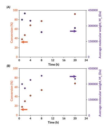
Fig. 3 Conversion and molar mass progression during US-mechanoredox *t*BA polymerizations under optimized conditions (see Table 3): (A) with BaTiO<sub>3</sub> (7 wt%) in DMF; (B) with ZnO (7 wt%) in DMAc.
