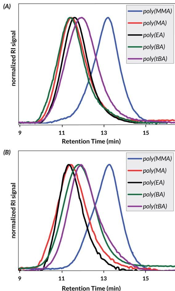
Fig. 2 GPC-RI traces of US-mechanoredox (meth)acrylate FRP using (A) BaTiO<sub>3</sub> or (B) ZnO as the PNP (see Table 3).
