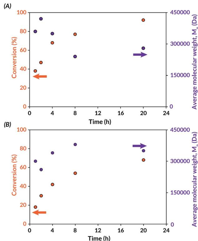
Fig. 3 Conversion and molar mass progression during US-mechanoredox *t*BA polymerizations under optimized conditions (see Table 3): (A) with BaTiO<sub>3</sub> (7 wt%) in DMF; (B) with ZnO (7 wt%) in DMAc.
