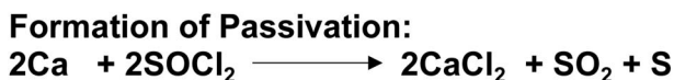
Fig. 2 Model for the formation of CaCl 2 passivation of the Ca metal in the Ca(AlCl 4 ) 2 -SOCl 2 electrolyte.
