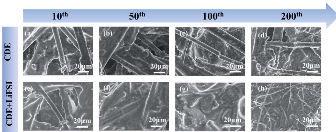
Fig. 6 SEM images of the carbon paper anode after cycling in CDE and CDE + LiFSI at the 10<sup>th</sup> (a and e), 50<sup>th</sup> (b and f), 100<sup>th</sup> (c and g) and 200<sup>th</sup> (d and h) cycles at 2C.
