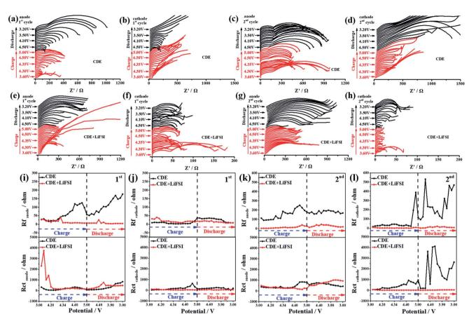
Fig. 5 In situ EIS profiles of Li-free CGDIBs on the cathode and anode at the first two cycles cycled in CDE (a-d) and in CDE + LiFSI (e-h). Variation trend plots of  $R_f$  and  $R_{ct}$  on the cathode and anode at the first two cycles cycled in CDE and CDE + LiFSI (i-l).
