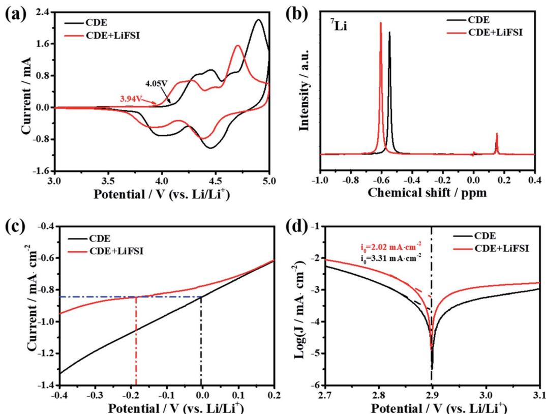
Fig. 2 (a) The CV curves of Li-free CGDIBs cycled in different electrolytes. (b)  $^7\text{Li}$  NMR spectra of different electrolytes. (c) LSV tests of Li deposition on a Pt electrode. (d) Tafel plots of different electrolytes.
