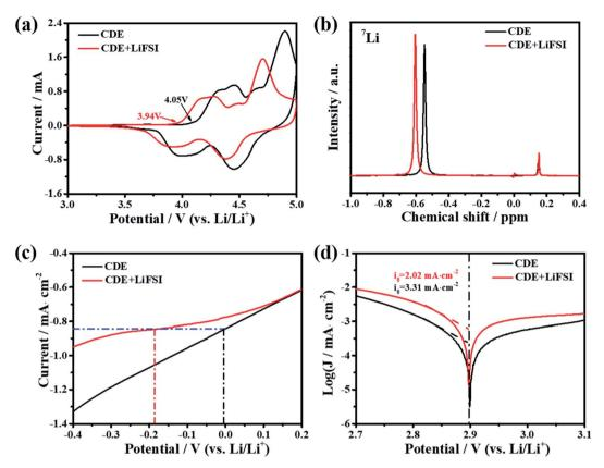
Fig. 2 (a) The CV curves of Li-free CGDIBs cycled in different electrolytes. (b) <sup>7</sup>Li NMR spectra of different electrolytes. (c) LSV tests of Li deposition on a Pt electrode. (d) Tafel plots of different electrolytes.
