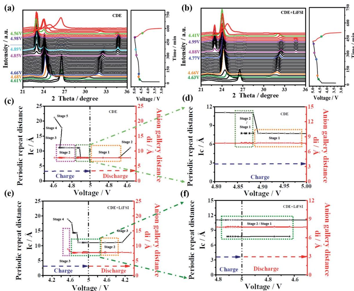
Fig. 7 *In situ* XRD spectra and the corresponding charge–discharge curves of Li-free CGDIBs during the first cycle in (a) CDE and (b) CDE + LiFSI. (c and e) The relevant change of periodic repeat distance  $I_c$  and the intercalated  $\text{PF}_6^-$  gallery height  $d_i$ . (d and f) The amplified plots of (c) and (e), respectively.
