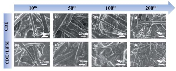
Fig. 6 SEM images of the carbon paper anode after cycling in CDE and CDE + LiFSI at the 10<sup>th</sup> (a and e), 50<sup>th</sup> (b and f), 100<sup>th</sup> (c and g) and 200<sup>th</sup> (d and h) cycles at 2C.
