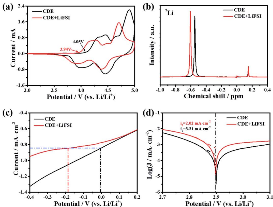
Fig. 2 (a) The CV curves of Li-free CGDIBs cycled in different electrolytes. (b)  $^7\text{Li}$  NMR spectra of different electrolytes. (c) LSV tests of Li deposition on a Pt electrode. (d) Tafel plots of different electrolytes.
