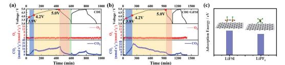
Fig. 3 OEMS tests of Li-free CGDIBs cycled in (a) CDE and (b) CDE + LiFSI at 0.5C for two cycles. (c) The DFT calculated structure and adsorption energy at the M06-L/(def2-SVP) level of theory.
