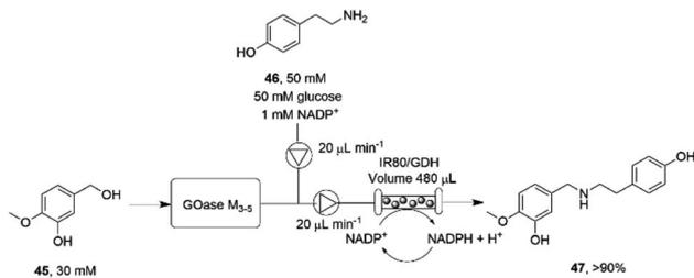
Scheme 18 Flow system for the oxidation-reductive amination cascade towards the synthesis of 4-*O*-methyl norbelladine **47**.<sup>77</sup>
