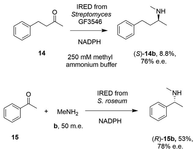
Scheme 4 Early examples of intramolecular asymmetric reductive amination reactions enabled by IREDs at high amine: ketone ratios.<sup>49,55</sup> (m.e. = molar equivalents). 'NADPH' in this and other schemes signifies the requirement of this reduced cofactor for the reaction, and is usually generated with the assistance of a cofactor recycling system comprising e.g. glucose dehydrogenase (GDH) and glucose, omitted from this and other schemes.
