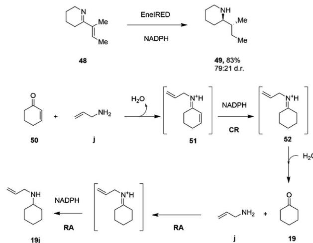
Scheme 19 Conjugate Reduction (CR) – Reductive Amination (RA) catalyzed by EneIRED.<sup>79</sup>
