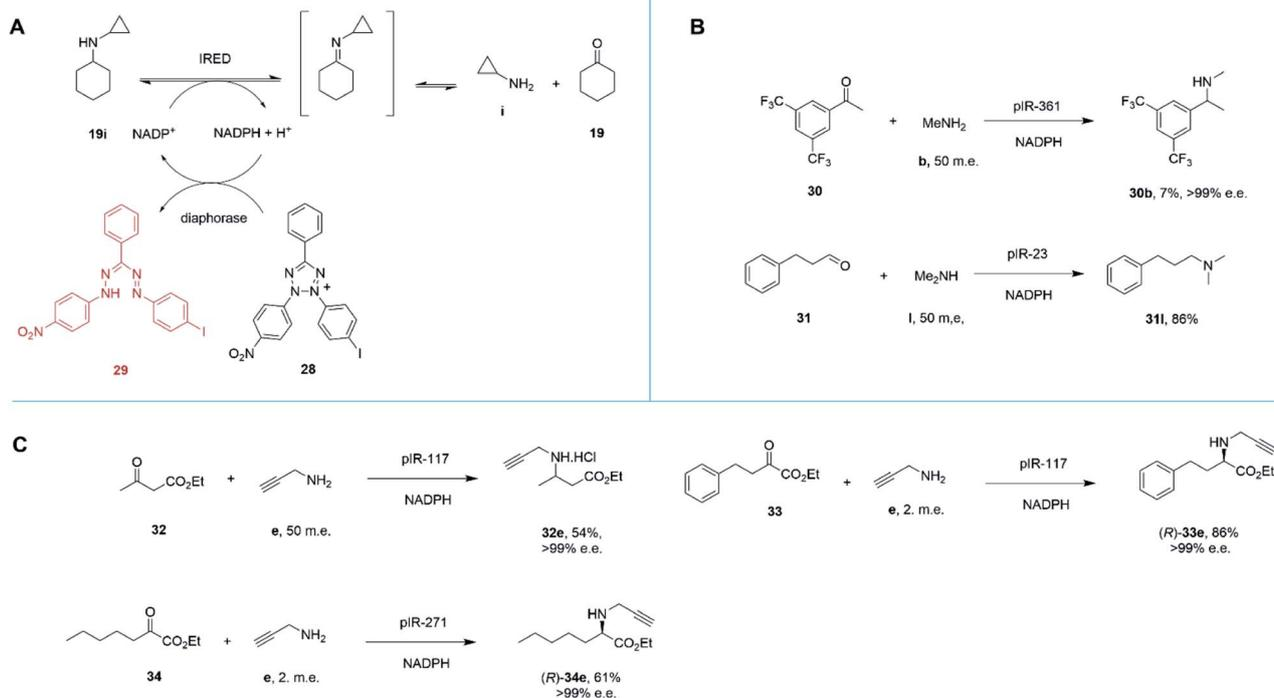
Scheme 13 (A) Chemical basis of IRED-y-to-go screen.<sup>68</sup> The oxidative activity of an IRED, acting on a secondary amine substrate, generates NADPH, which is used by diaphorase to reduce tetrazolium salt **28** to red dye **29**. (B) The IRED-y-to-go screen was used to identify IREDs that enabled aminations of acetophenones **30** and the production of tertiary amines.<sup>68</sup> (C) The IRED-y-to-go screen enabled also identified enzymes for the amination of esters.<sup>68,69</sup>
