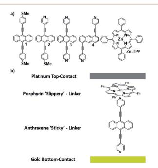
Fig. 1 (a) Chemical structures of studied molecules; (b) typical schematic of a fabricated junction.
