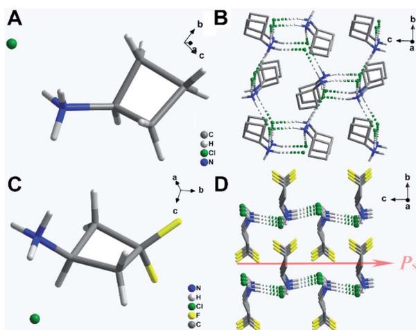
Fig. 2 Crystal structures of (CBA)Cl and (3,3-DFCBA)Cl. The structural unit of (CBA)Cl (A) and (3,3-DFCBA)Cl (C) at 293 K. Packing views of (CBA)Cl (B) and (3,3-DFCBA)Cl (D) along the  $a$ -axes at 293 K. Hydrogen atoms were omitted for clarity. The green dashed lines stand for the N–H $\cdots$ Cl hydrogen bonding interactions. The direction of spontaneous polarization of (3,3-DFCBA)Cl is shown with the red arrow.
