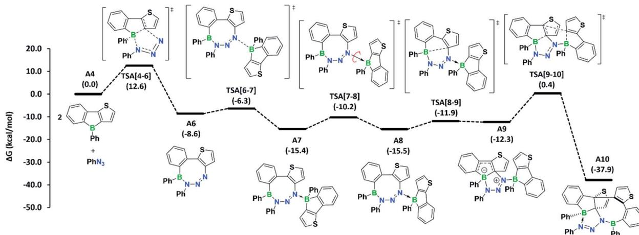
Fig. 4 Mechanism computed for azide adduct formation at the B3LYP-D3BJ/6-311g+\*\*/SMD(C<sub>6</sub>H<sub>6</sub>)//B3LYP-D3BJ/6-31g\*\* level of theory. Free energies in parentheses are in kcal mol<sup>-1</sup>.
