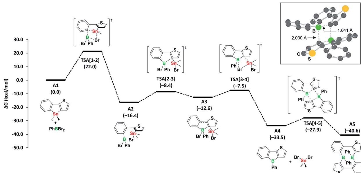
Fig. 2 Computed mechanism for diborocycle formation *via* tin–boron exchange. Free energies in parentheses are in kcal mol<sup>-1</sup>. DFT-optimised structure with key distances of the transition state responsible for the borole-to-diborocycle interconversion (TSA[4-5]) is shown in the inset in the top right corner.
