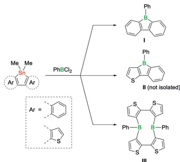
Scheme 1 Products of the tin–boron exchange reaction of fused stannoles with  $\text{PhBCl}_2$ , according to He *et al.*<sup>6</sup>
