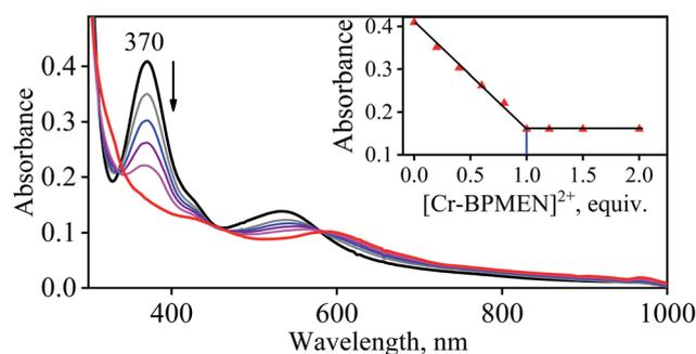
**Fig. 4** UV-Vis spectral changes observed in the reaction **1-CoNO** with **2-Cr** (in the increments of 0, 0.20, 0.40, 0.60, 0.80, 1.0, 1.2, 1.5, 2.0 equivalent) in  $\text{CH}_3\text{CN}$  under Ar at 298 K.
