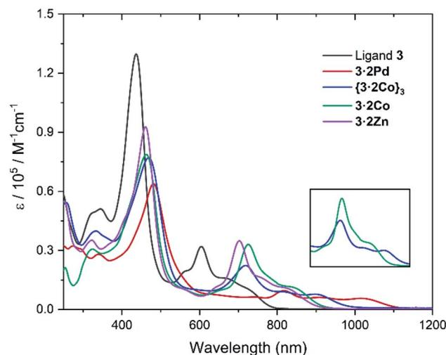
Fig. 6 UV-vis-NIR absorption spectra of ligand **3**,  $3 \cdot 2\text{Pd}$ ,  $\{3 \cdot 2\text{Co}\}_3$ ,  $3 \cdot 2\text{Co}$ , and  $3 \cdot 2\text{Zn}$  in  $\text{CHCl}_3$  at room temperature. (inset) Comparative of  $\{3 \cdot 2\text{Co}\}_3$  and  $3 \cdot 2\text{Co}$  expanded region at 600–1000 nm.
