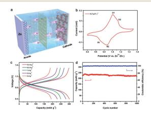
Fig. 3 (a) Illustration of the aqueous Zn/Tp-PTO-COF battery; (b) CV curve at a scan rate of 0.5 mV s $^{-1}$ ; (c) galvanostatic charge–discharge curves of the aqueous Zn/Tp-PTO-COF battery at various current densities; (d) cycle stability at a current density of 2 A g $^{-1}$ .
