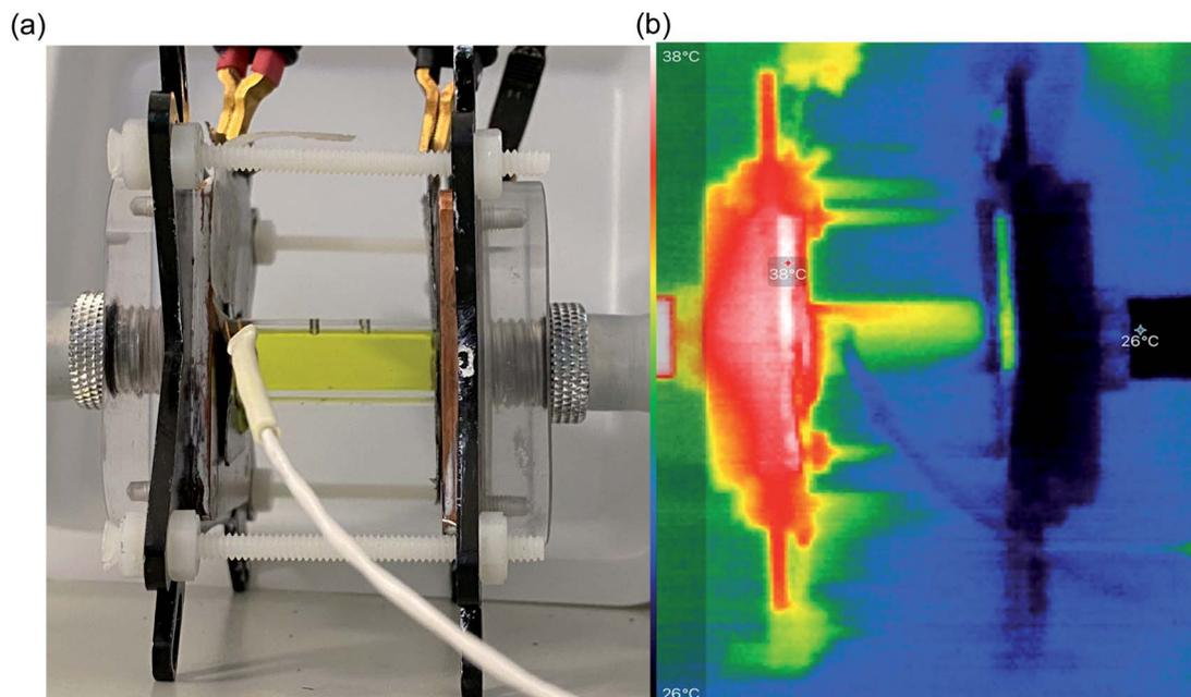
Fig. 4 Photos of (a) the actual thermogalvanic cell, sandwiched between the two heat exchangers (the white wire coming from the left is the heat flux sensor wiring); electrode separation = 29.3 mm,  $\Delta T_{\text{app}} = 20$  K; and (b) IR image of the same cell, going from white = hottest to black = coldest.
