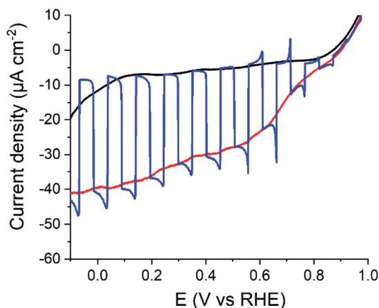
Fig. 5 LSVs at FTO/NiO/[P3HT:PCBM+**1**] electrode with (red line), without (black line) or with chopped (blue line) visible light ( $400 < \lambda < 800 \text{ nm}$ ,  $65 \text{ mW cm}^{-2}$ ) recorded at a scan rate of  $5 \text{ mV s}^{-1}$  in  $0.1 \text{ M}$  acetate buffer (pH 4.5).
