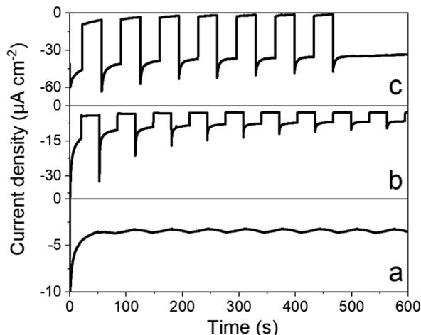
Fig. 6 Photocurrent densities measured under chopped visible light ( $400 < \lambda < 800\text{ nm}$ ,  $65\text{ mW cm}^{-2}$ ) at an applied potential of  $0.065\text{ V vs. RHE}$  in  $0.1\text{ M acetate buffer (pH 4.5)}$  for the following electrodes: FTO/NiO (a), FTO/NiO/P3HT:PCBM (b) and FTO/NiO/[P3HT:PCBM+1] (c).
