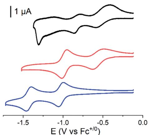
Fig. 2 Cyclic voltammograms for **nmep-pC<sub>60</sub>** (blue), **2** (red) and **1** (black), recorded in a 0.3 mM CH<sub>3</sub>CN/1,2-dichlorobenzene 1 : 1 (v/v) solution in the presence of 0.1 M of *n*-Bu<sub>4</sub>NBF<sub>4</sub> on glassy carbon (∅ 1.6 mm); scan rate: 100 mV s<sup>-1</sup>. All measurements were started after equilibration at the open-circuit potential around –0.1 V *vs.* Fc<sup>+0</sup>/Fc with initial scan towards more negative potentials.
