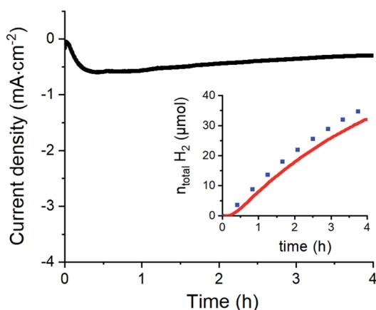
Fig. 4 Long-term chronoamperometric experiment at  $-0.63 \text{ V vs. RHE}$  in acetate buffer ( $0.1 \text{ M}$ , pH 4.5) with concomitant  $\text{H}_2$  quantification (red trace in inset); the blue dots indicate the expected  $\text{H}_2$  amount for a  $100\%$  faradaic yield.
