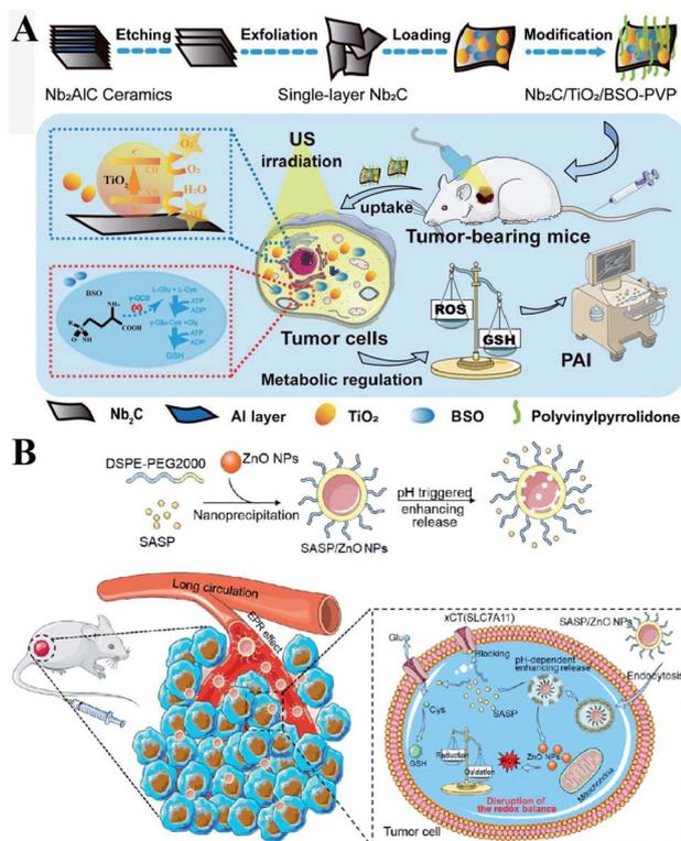
Fig. 9 (A) Schematic illustrations of the synthesis process and function of the Nb<sub>2</sub>C/TiO<sub>2</sub>/BSO-PVP. Adapted from ref. 49 with permission. Copyright 2020 Wiley-VCH. (B) Design and application of SASP/ZnO NPs for cancer therapy. Adapted from ref. 53 with permission. Copyright 2019 American Chemical Society.
