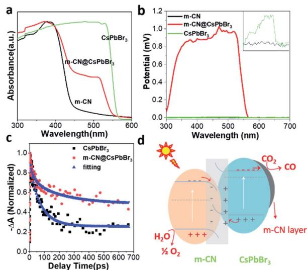
Fig. 2 (a) UV-Vis absorption spectra of m-CN@CsPbBr<sub>3</sub>, the reference m-CN and CsPbBr<sub>3</sub>; (b) surface photovoltage plots of the m-CN, CsPbBr<sub>3</sub> and m-CN@CsPbBr<sub>3</sub> samples; (c) transient absorption spectroscopy curves and lifetime fittings at 520 nm; (d) band structure of the m-CN@CsPbBr<sub>3</sub> heterojunction and the corresponding paths of CO<sub>2</sub> photo-reduction.
