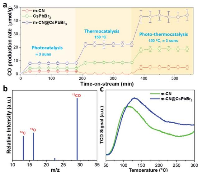
Fig. 3 (a) The CO<sub>2</sub> reduction to CO performance under the three conditions of photocatalysis, thermocatalysis and photo-thermocatalysis. For the latter two, the temperature is set to 150 °C; (b) mass spectrometry (MS) result of <sup>13</sup>CO produced over m-CN@CsPbBr<sub>3</sub> from the <sup>13</sup>CO<sub>2</sub> isotope experiment under thermocatalysis (*m/z*, mass/charge ratio); (c) CO<sub>2</sub>-TPD results of the reference m-CN and the m-CN@CsPbBr<sub>3</sub> catalyst.
