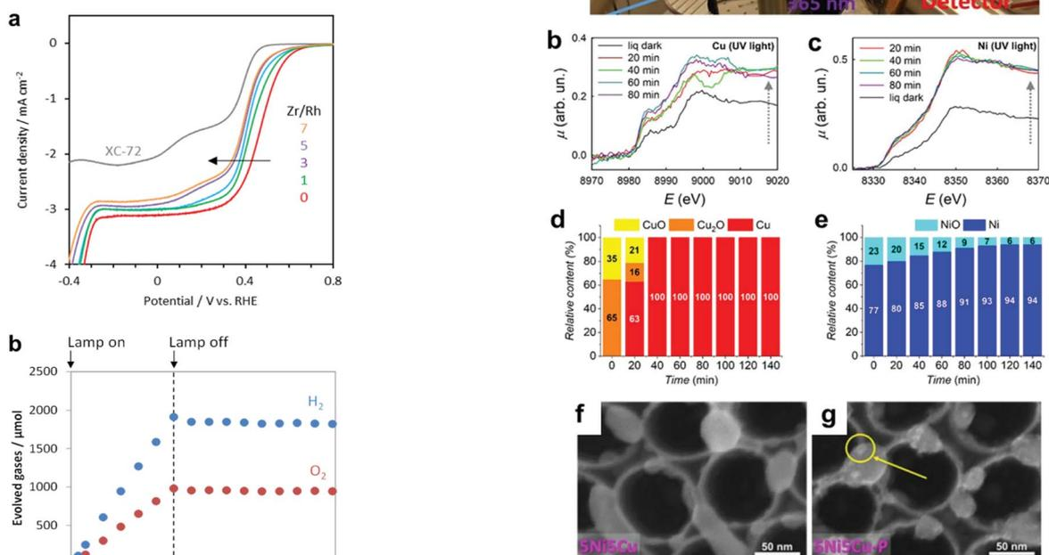
Fig. 12 (a) Current–potential curves of  $\text{RhZrO}_x$  (Zr/Rh: 0–7 w/w)-loaded carbon supports in  $\text{O}_2$ -saturated 1 M  $\text{Na}_2\text{SO}_4$  (pH 7); (b) gas evolution over time by  $\text{RhZrO}_x/\text{SrTiO}_3:\text{Al}$  (Rh = 0.1 wt% and Zr = 0.5 wt% vs.  $\text{SrTiO}_3:\text{Al}$ ) during and after light irradiation (300 W Xe lamp). Adapted with permission from ref. 169; copyright 2020 RSC.
