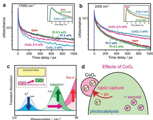
Fig. 10 Decay of transient absorption at (a)  $17\,000\text{ cm}^{-1}$  and (b)  $2000\text{ cm}^{-1}$  for bare,  $\text{CoO}_x$ -loaded, and Pt-loaded  $\text{LaTiO}_2\text{N}$  after excited by 500 nm laser pulses; (c and d) schematics showing the change in carrier dynamics upon  $\text{CoO}_x$  CC loading. Adapted with permission from ref. 157; copyright 2014 ACS.
