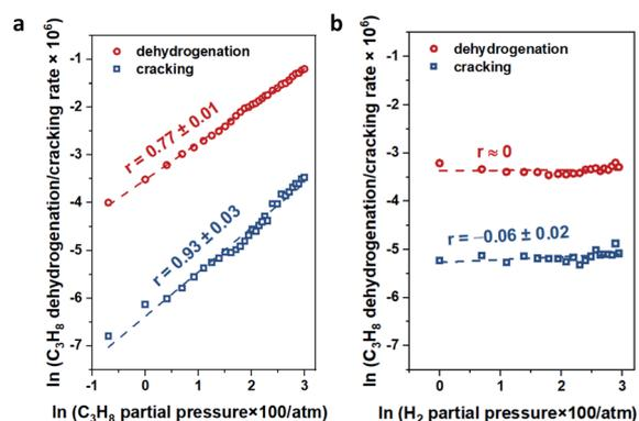
Fig. 11 The dependence of propane dehydrogenation and cracking reactions on (a) propane partial pressure and (b) H<sub>2</sub> partial pressure over the In-CHA(11, 1.0) catalyst at 600 °C.
