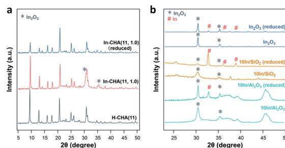
Fig. 1 XRD patterns of samples investigated after calcination and reduction: (a) H-CHA(11) and In-CHA(11, 1.0); (b) indium on silica and alumina and bulk  $\text{In}_2\text{O}_3$ . The diffraction peaks at  $2\theta$  values of  $30.6^\circ$  and  $35.5^\circ$  (marked with asterisks) are assigned to  $\text{In}_2\text{O}_3$  (JCPDS 060416), and diffraction peaks at  $2\theta$  values of  $33.0^\circ$ ,  $36.3^\circ$  and  $39.2^\circ$  (marked with #) are associated with In(0) (JCPDS 05-0642).
