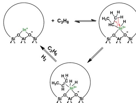
Scheme 1 Schematic of proposed mechanisms for PDH on isolated In<sup>+</sup> sites.
