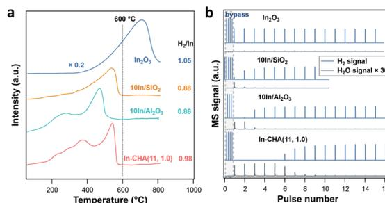
Fig. 2 (a) H<sub>2</sub>-TPR profiles and (b) results of H<sub>2</sub> pulse experiments on In-based catalyst at 600 °C.
