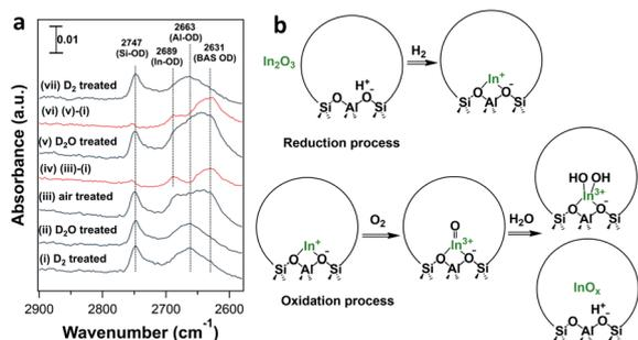
Fig. 8 (a) FTIR spectra of reduced In-CHA(11, 1.0) treated under different conditions at 550 °C: (i) D<sub>2</sub>; (ii) D<sub>2</sub>O; (iii) air; (iv) (i) subtracted from the spectrum (iii); (v) D<sub>2</sub>O; (vi) (i) subtracted from the spectrum (v); (vii) D<sub>2</sub>O. Background spectrum was collected in the spectral cell with the H<sub>2</sub> reduced sample pellet at 550 °C. (b) Proposed structures of exchanged In species in In-CHA upon reduction and subsequent oxidation.
