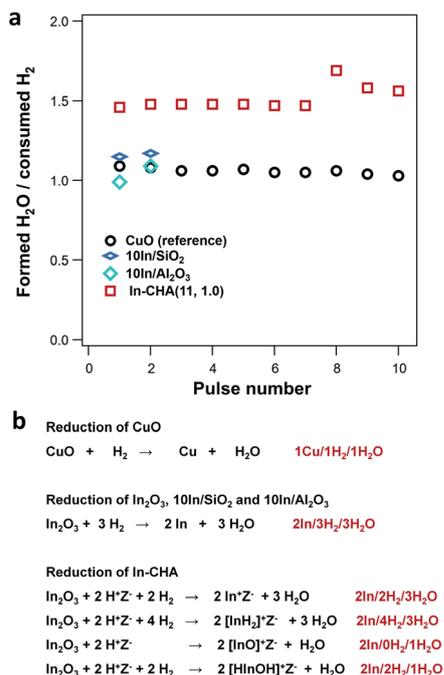
Fig. 3 (a) Determination of the formed H<sub>2</sub>O/consumed H<sub>2</sub> ratio from H<sub>2</sub> pulses as a function of pulse number on several catalysts. (b) Stoichiometric analysis during reduction on CuO, In<sub>2</sub>O<sub>3</sub>, 10In/SiO<sub>2</sub>, and 10In/Al<sub>2</sub>O<sub>3</sub>, and potential reactions on In-CHA catalysts.
