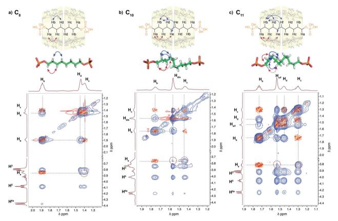
Fig. 5 Stack between the COSY (red) and NOESY (blue) NMR spectra (600 MHz,  $D_2O$ , pH = 10) of [3] pseudorotaxane with (a)  $C_8$ , (b)  $C_{10}$ , and (c)  $C_{11}$  axles and optimized geometries of axles in the corresponding [3] rot. Long range NOE correlations  $H_a - H_{d/e}$  and  $H_b - H_{d/e}$  and  $H_b$
