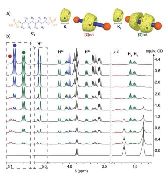
Fig. 3 (a) Equilibrium of formation of [2] and [3] pseudorotaxanes with the  $C_8$  axle. (b)  $^1H$  NMR (600 MHz,  $D_2O$ , 300 K) titration of the  $C_8$  axle (2.8 mM) with CD in acetate buffer at pH = 5 showing the progressive appearance of [2] rot (red), [3] rot (green) and free CD (blue).
