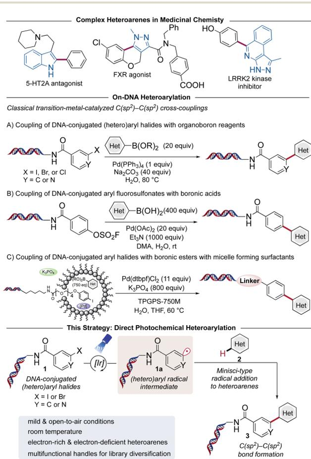
**Scheme 2** Medicinally relevant heteroarene scaffolds containing (hetero)arene  $C(sp^2)$ – $C(sp^2)$  bonds (top). On-DNA heteroarylation protocols using palladium two-electron cross-coupling processes (middle). This strategy: direct photochemical C–H heteroarylation through the intermediacy of aryl radicals (bottom).
